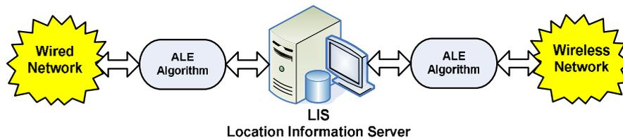
**Fig. ( 2): Different Types of ALEs for Different Access Networks**
