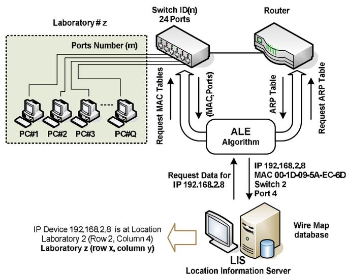
**Fig. ( 6 ) : Static IP Assignments Using ARP Table Location Determination System**
