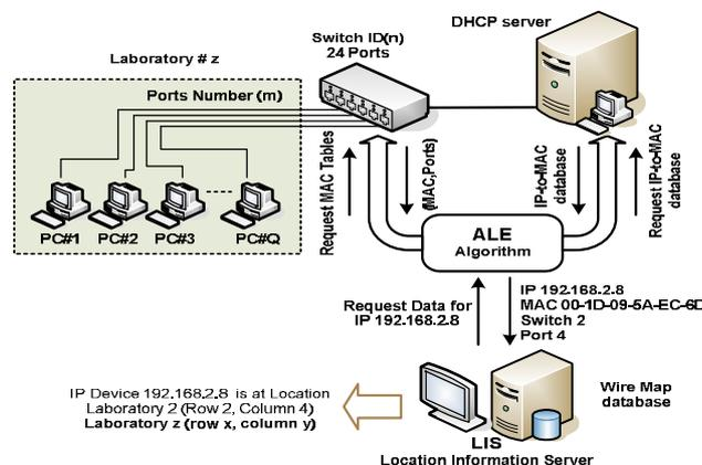
**Fig. ( 8 ) : Dynamic IP Assignments Location Determination System**
