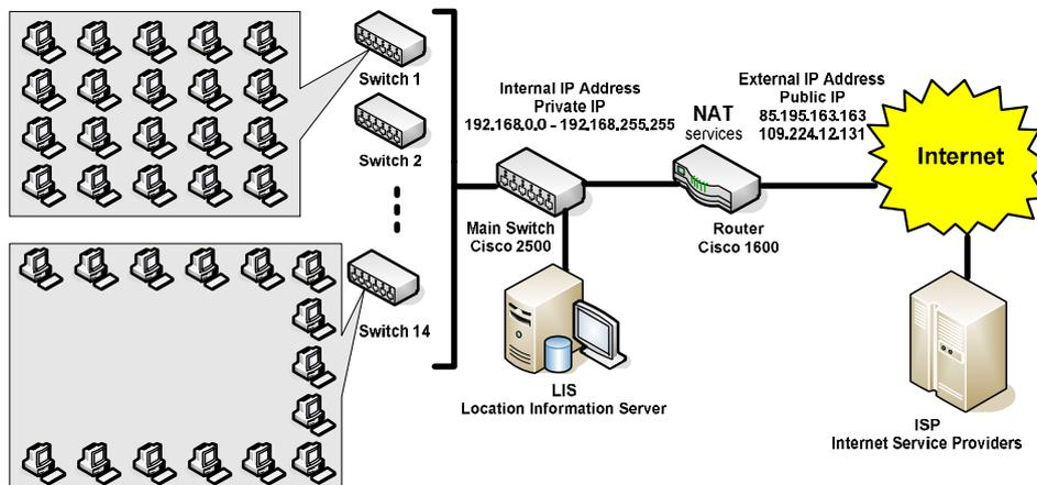
**Fig. ( 4): The Network Structure of Computer Center with IP Addressing Scheme**
