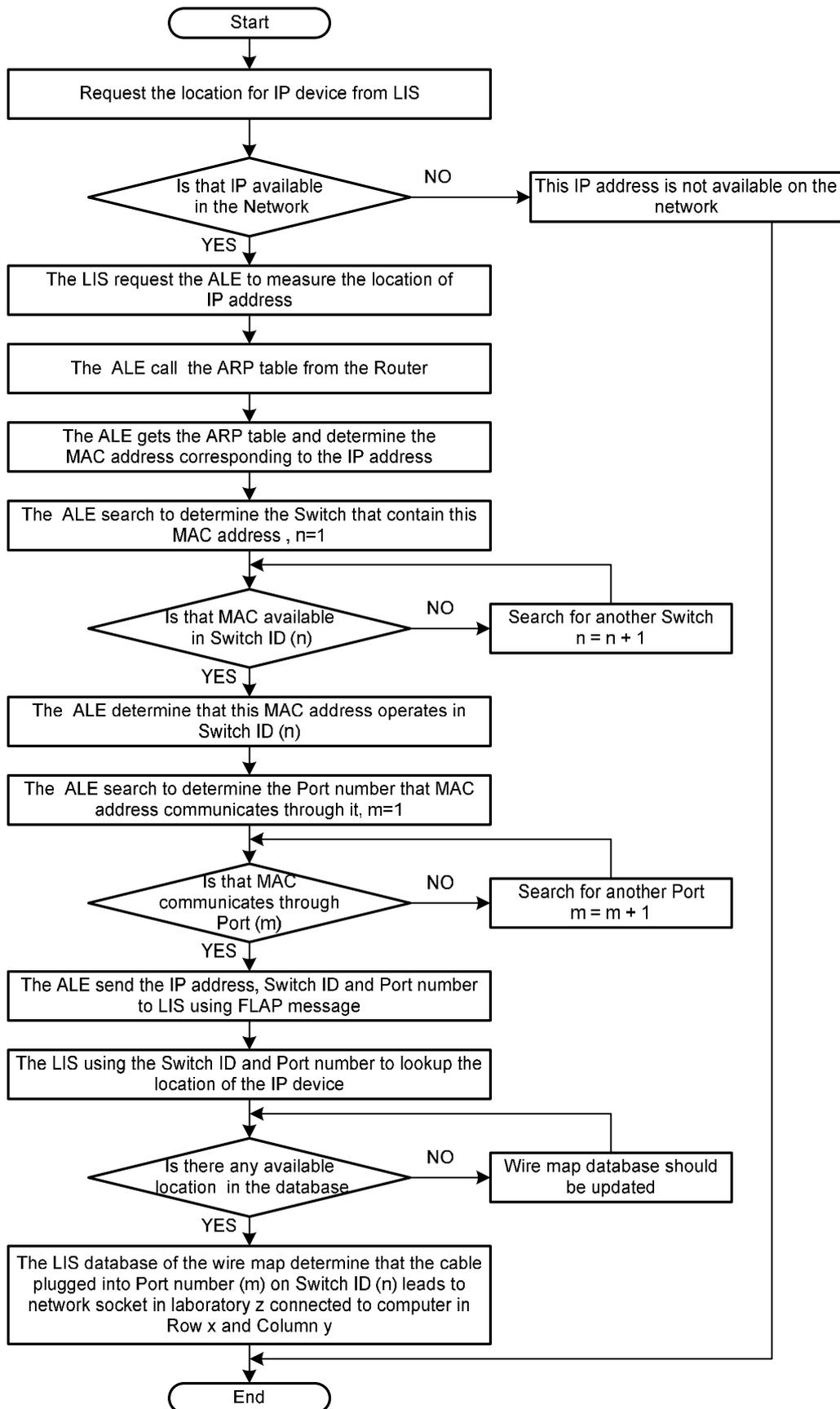
**Fig. (7) : Flowchart Explains Static IP Assignments Location Determination System**
