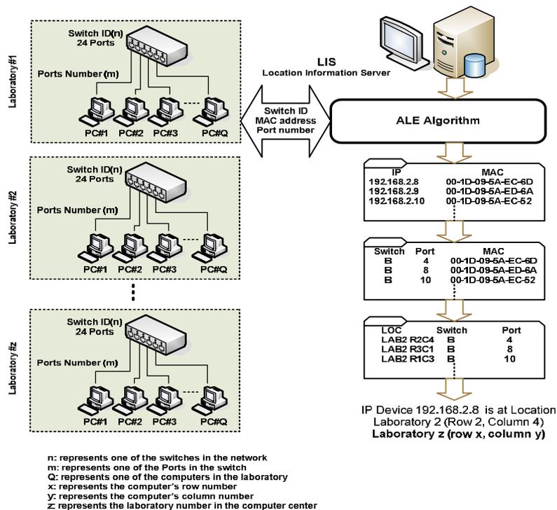
**Fig. (5): Location Determination Using IP to MAC,MAC to Switch and Switch to Port Chain**
