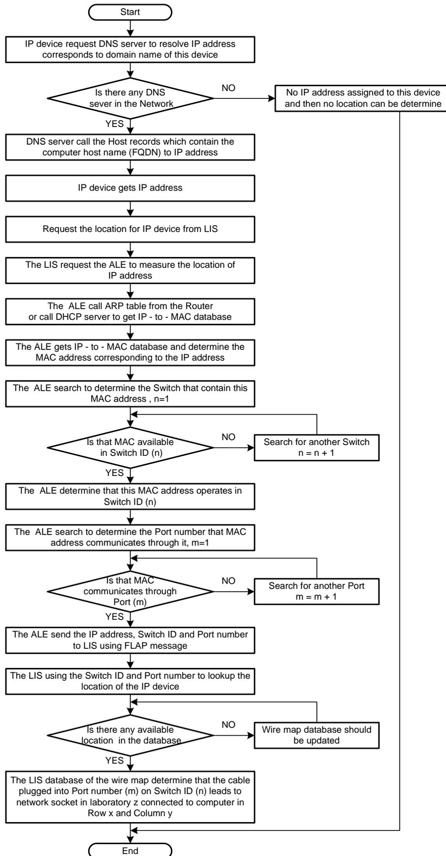
**Fig. (11): Flowchart Explains Domain Name System Based Location Determination System**
