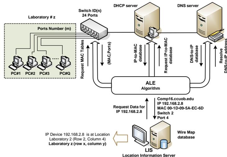
**Fig. (10) : Domain Name System Based Location Determination System**
