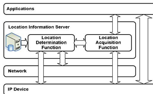
**Fig. (1) : Location Determination System Architecture**
