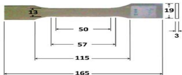
**Fig.(2-1) the polyester specimen <sup>[11]</sup> (Dimensions are in mm)**
