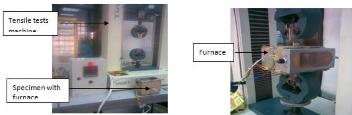
**Fig. (2-3) a-Specimen with the Furnace      b- Specimen Fixture with the Furnace**
