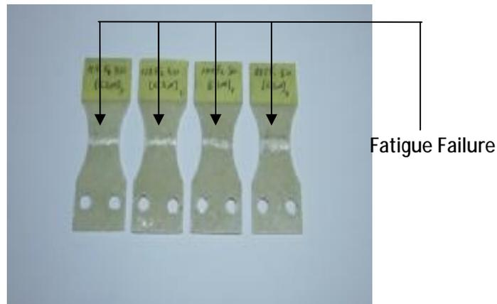
**Figure (3-3) Fatigue Failure of Composite Specimens**
