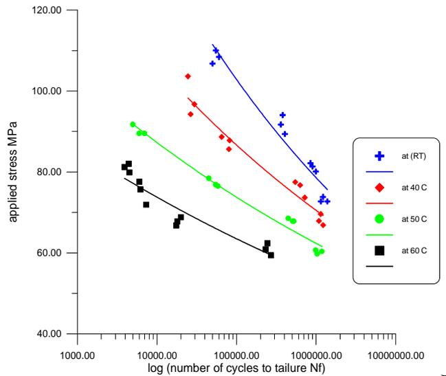
**Fig. (3-2) S-N curve for [CSM]<sub>3</sub> laminate at different temperature**
