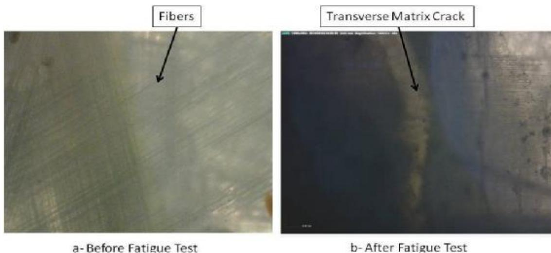
**Figure (3-4) micrographs of fatigue failure observed in polyester-E glass composite (40X)**
