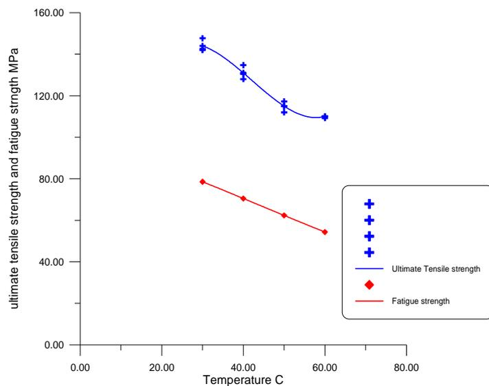
**Fig. (3-1) fatigue strength and ultimate tensile strength at different temperature for laminate**
