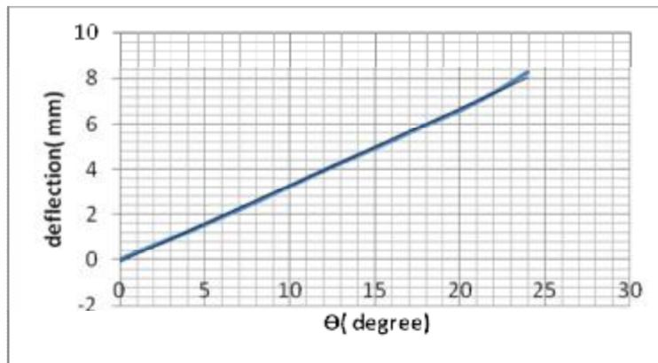
Fig. (A-3)) calibration curve between bending deflection and eccentric position angle ( $\Theta$ )
