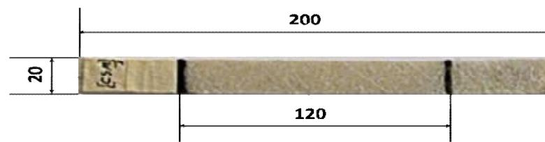
**Fig. (2-2) tensile test specimen dimensions (Dimensions are in mm)**
