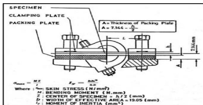
Fig. (A-1) Schematic Representation of Fixing Method, And how to Calculate Bending stress [13]
