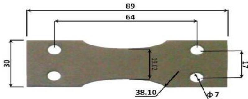
Fig. (2-5) Fatigue Specimens (all dimension in mm) [14]
