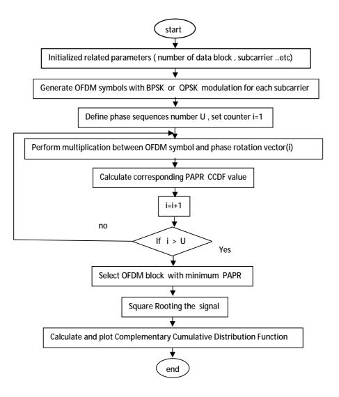
Fig. (3) propose transmitter flowchart .
