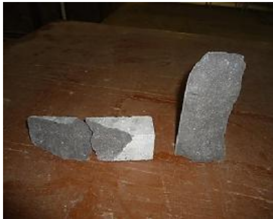
Fig.(14-a) Explosive spalling of wet RPC-0% at 400°C.
