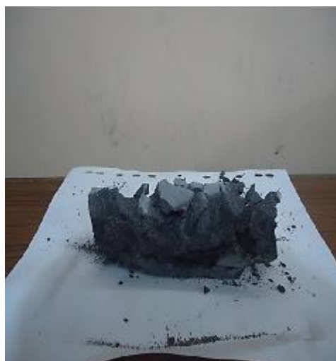
Fig. (15-a) Explosive spalling of wet RPC-1% at 600°C
