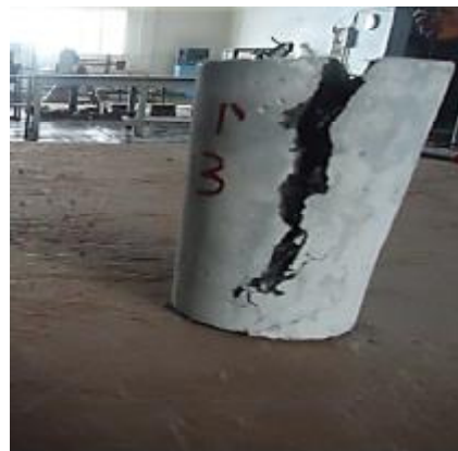
Fig.(14-d) Explosive spalling of wet RPC-3% at 400°C
