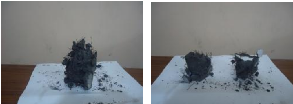
Fig.(15-b) Explosive spalling of wet RPC-2% at 600°C
