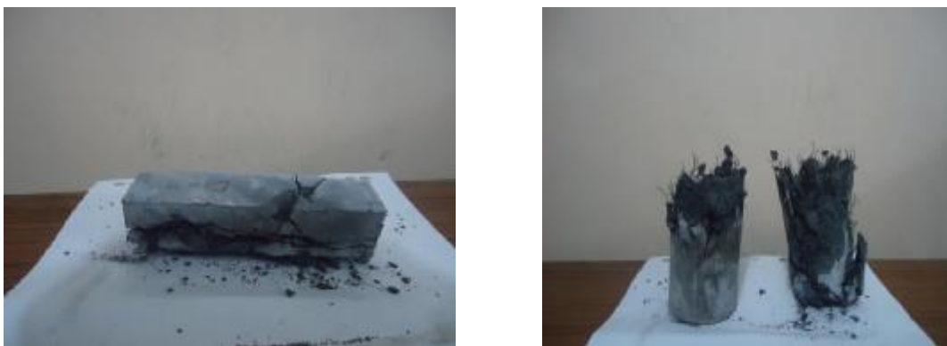
Fig. (15-c) Explosive spalling of wet RPC-3% at 600°C
