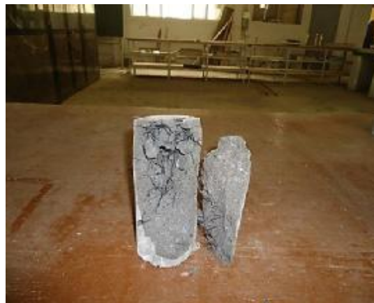
Fig. (14-b) Explosive spalling of wet RPC-1% at 400°C
