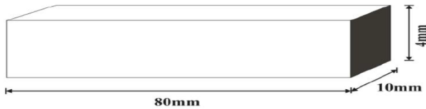
Figure 8. Dimension of the specimen impact
