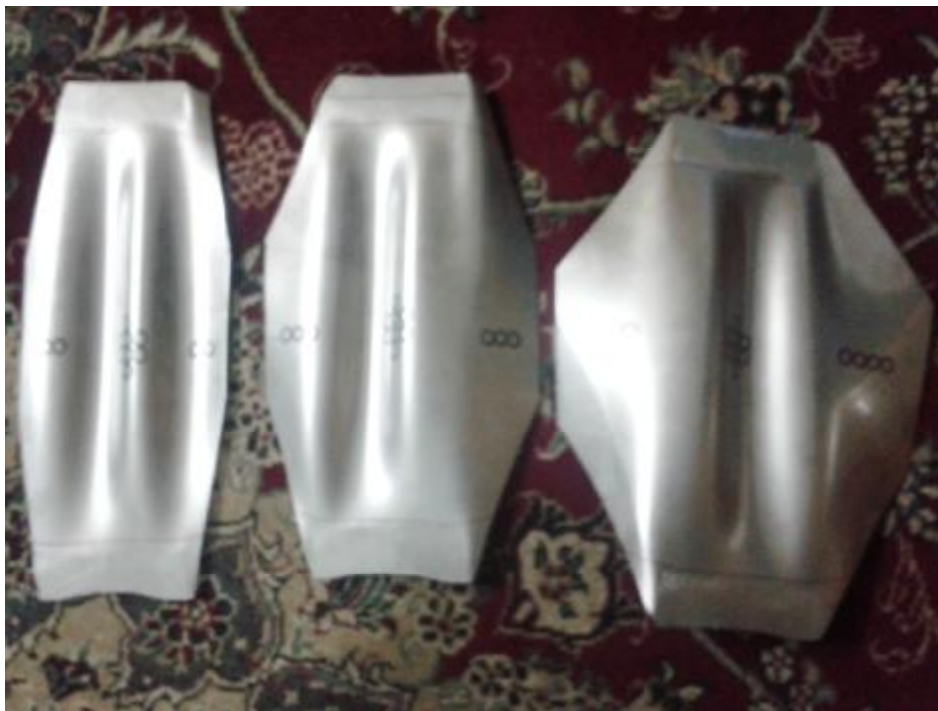
Fig.(9) Image of specimen after deformation of buckling
