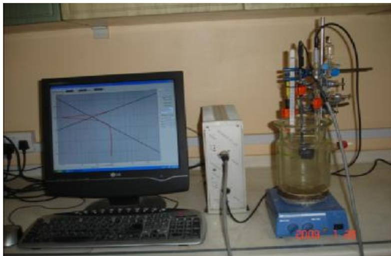
**Fig. (2) the electrochemical corrosion unit**
