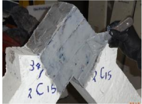
(b) Resin Applied to the knee joint
