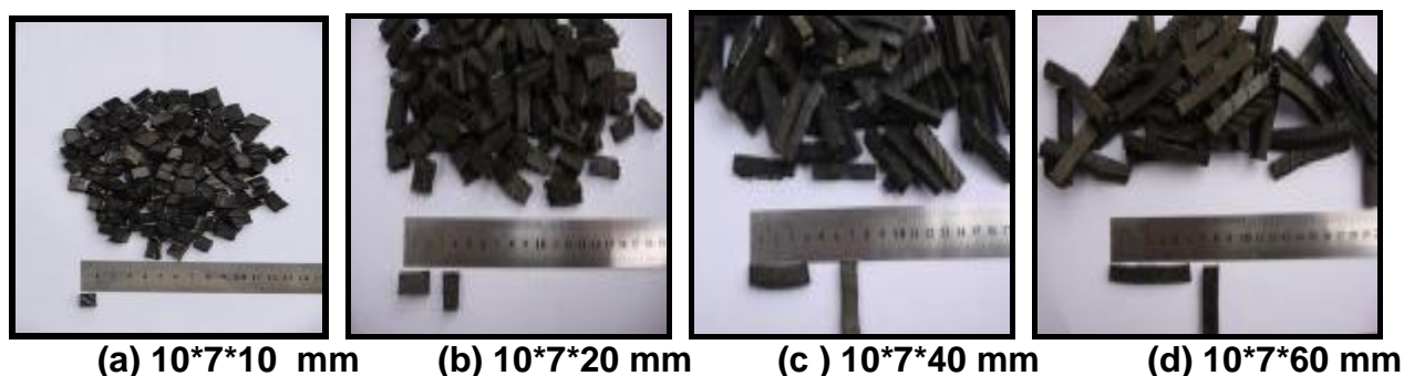
plate (2) Rubber Strips and Chips Dimensions
