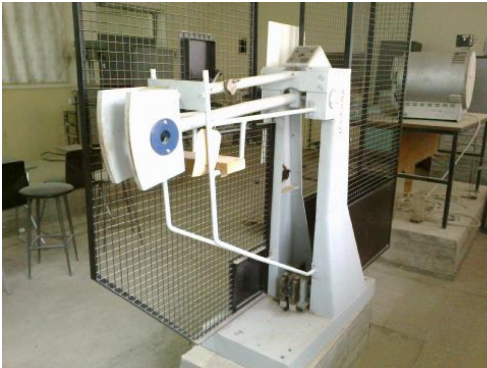
Fig. (3) Image of equipment for impact
