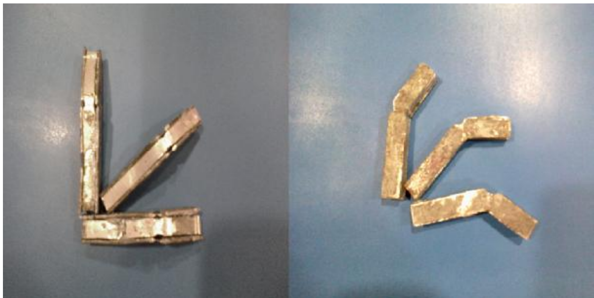
Fig. (16) image of sandwich specimens after impact
