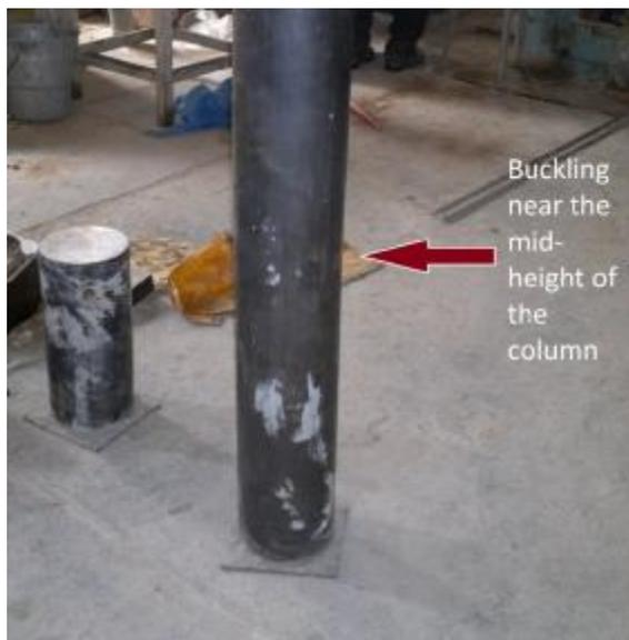
Fig.( 7) Failure of the long column.
