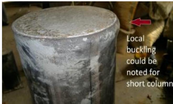
**Fig. (4) Failure of the short column.**
