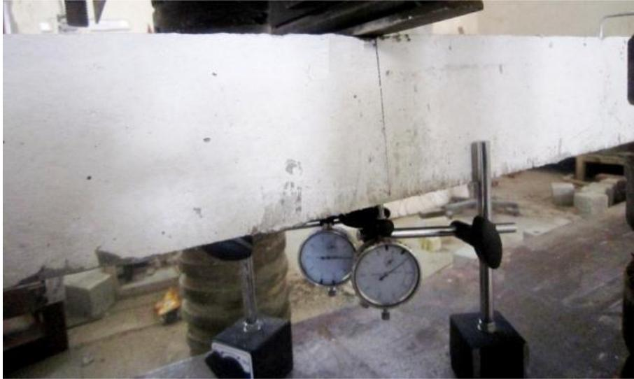
**Plate (1) Two Dial Gauges are Below the Center of Beams**
