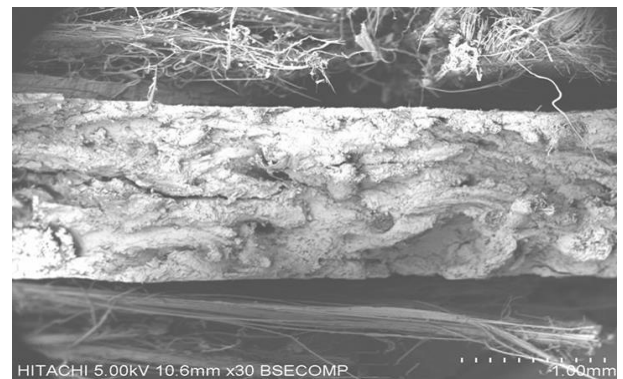
Figure 4. Delamination of Impact Specimen (40%) under SEM Micrograph.
