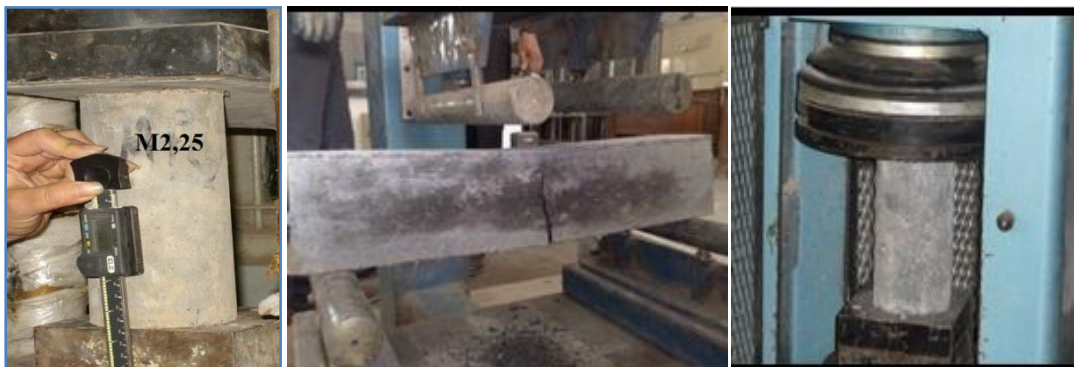
Plate .(3) Modulus of Elasticity ( E_o ), Modulus of Rupture and Compressive Strength ( f'_{cf} ) Tests
