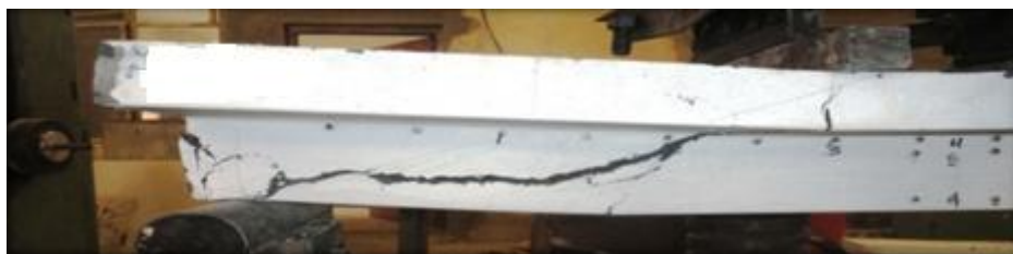
Plate .(4): Shear Failure Mechanism of Simply Supported in RPC T- Beam.
