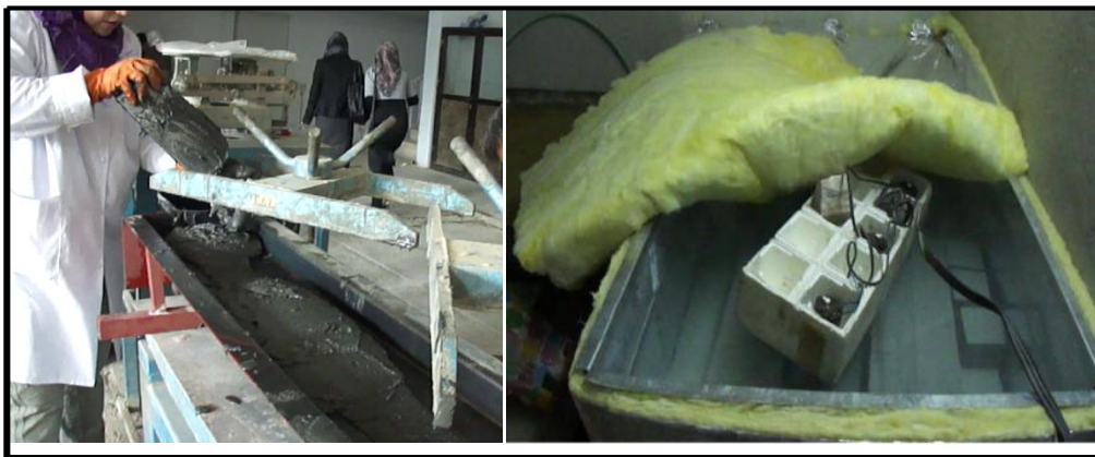
Plate (1) casting and curing of specimens
