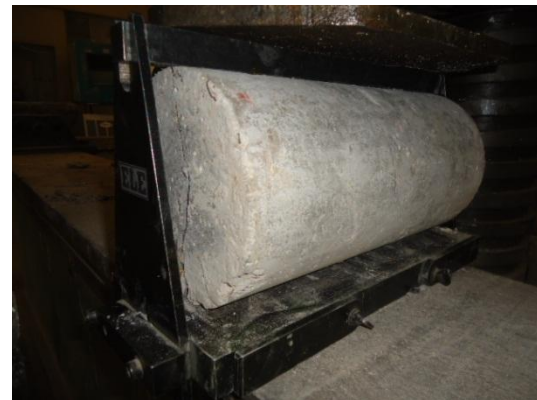
Fig .(16) Splitting failure of fibrous HSCC cylinder
