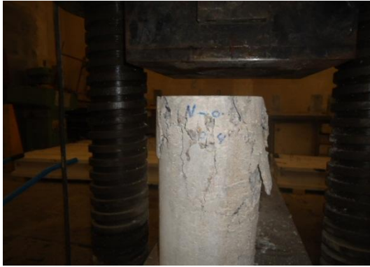
Fig .(9) Failure of NSCC cylinders with steel fibers
