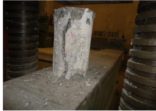
Fig .(10) Failure of HSCC cylinders with steel fibers
