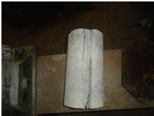
Fig .(15) Splitting failure of fibrous NSCC cylinder
