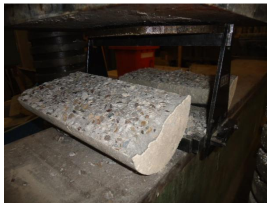
Fig .(13) Splitting failure of nonfibrous NSCC cylinder
