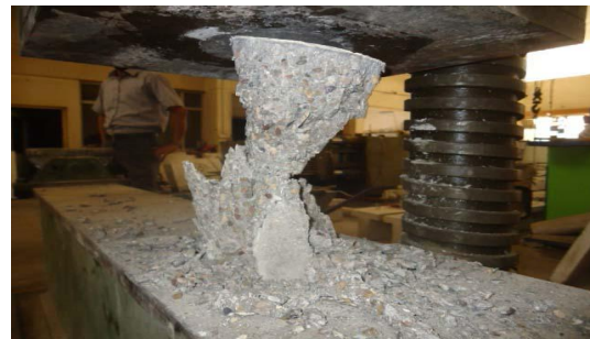
Fig .(8) Failure of HSCC cylinders without steel fibers
