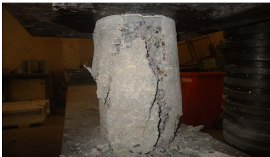
Fig .(7) Failure of NSCC cylinders without steel fibers
