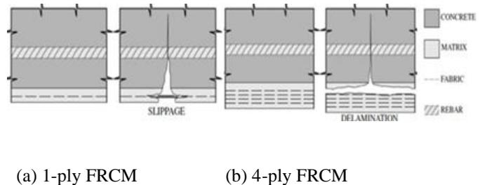
**Figure 4.** Schematic of the 1-ply and 4-ply FRCM-reinforced RC-beam failure mode [65]
