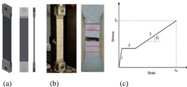
**Figure 3.** (a) Dumbbell TRM voucher; (b) rupture of the fibers; (c) the relationship of stress and strain vs for TRM specimens subjected to monotonic tensile [54].
