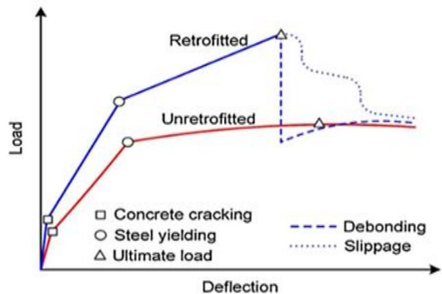
Figure 2. Strengthening effect of RC members in flexure [3]
