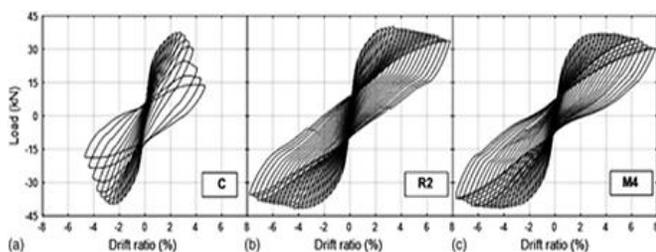
**Figure 6.** Curves relating load to the percentage of drift for a) the normative sample, b) The FRP-restricted specimen, and c) The specimen restricted by TRM [7].
