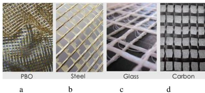
**Figure 1.** Textile fiber types: (a) polyphenylene bezobisoxazole (PBO); (b) steel fiber textile; (c) glass fiber textile; and (d) carbon fiber textile [8]
