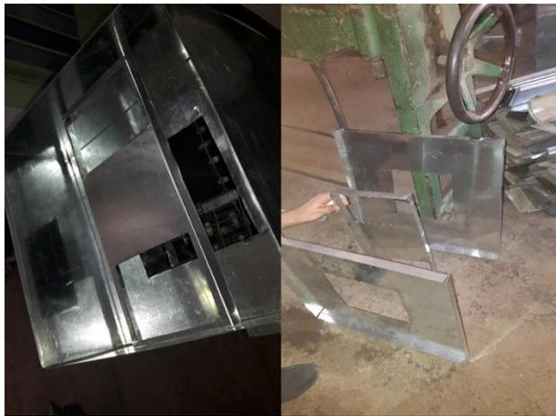
Figure 4. Mixing Baffles
