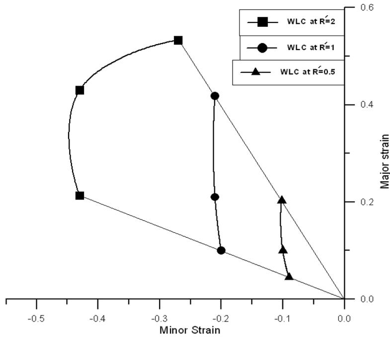
**Fig .(7) Effect of normal plastic anisotropic ratio on WLC**
