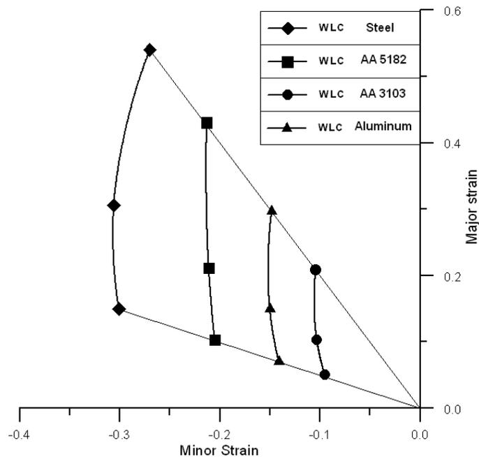
**Fig .(11) Comparison of wrinkling limit curve between the steel, aluminum and aluminum alloy(AA 3103, AA 5182) sheets**
