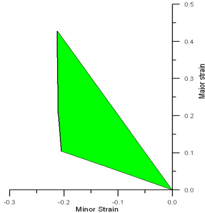
**Fig .(5) Wrinkling limit diagram of Aluminum alloy AA5182 sheet**
