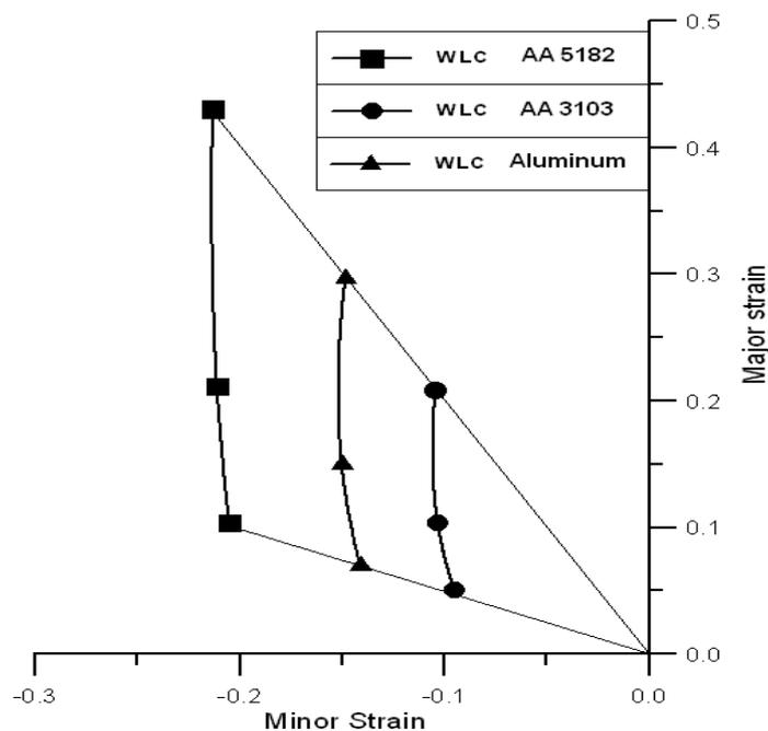
**Fig .(10) Comparison of wrinkling limit curve between the aluminum and aluminum alloy(AA 3103, AA 5182) sheets**
