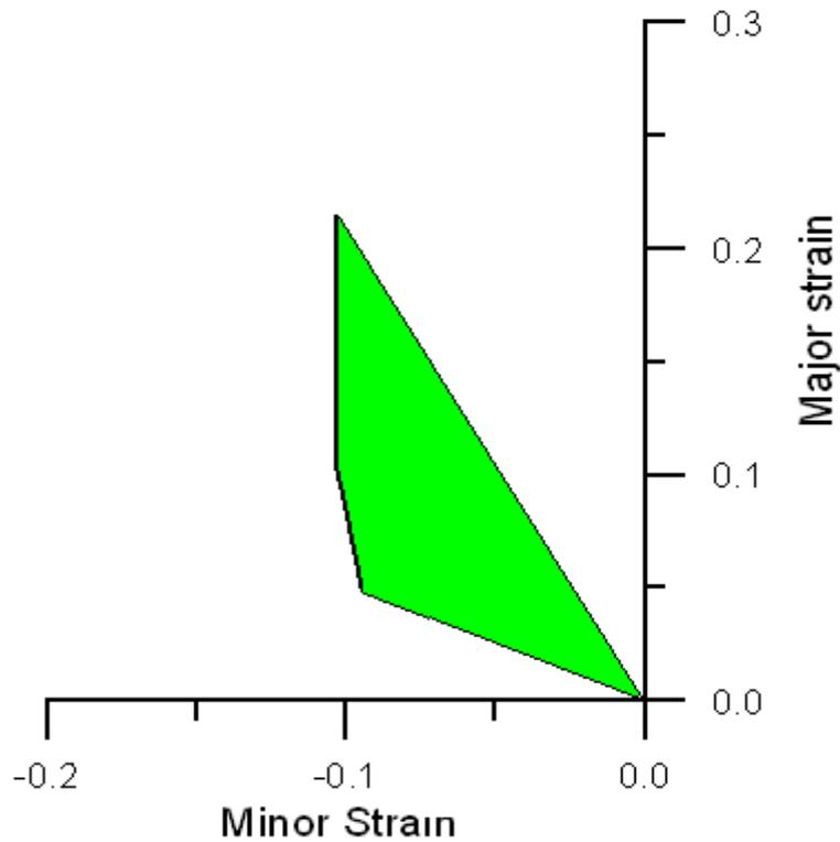
**Fig .(4) Wrinkling limit diagram of Aluminum alloy AA3103 sheet**
