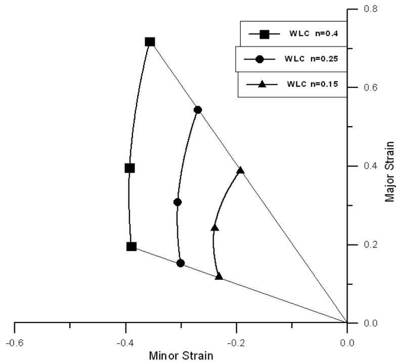
**Fig .(6) Effect of strain hardening exponent on WLC**
