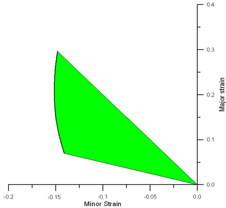
**Fig .(3) Wrinkling limit diagram of Aluminum sheet**
