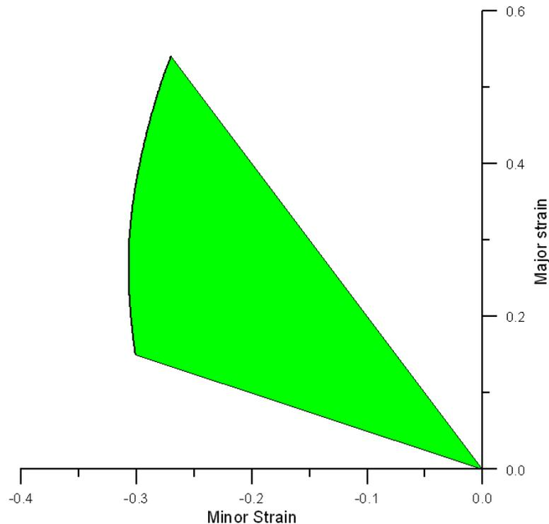
**Fig .(2) Wrinkling limit diagram of Steel sheet**
