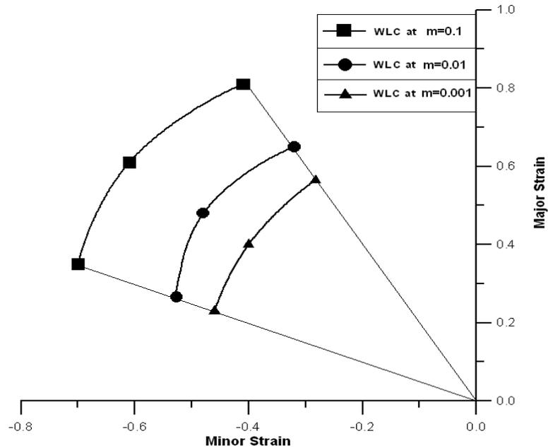
**Fig .(9) Effect of Strain rate sensitivity exponent on WLC**
