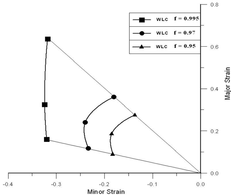
**Fig .(8) Effect of imperfection factor on WLC**
