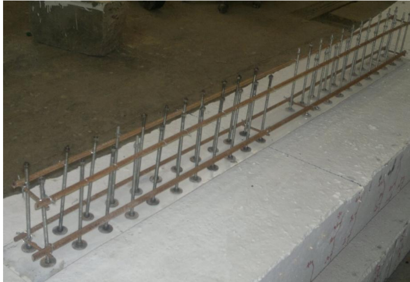
Fig .(2) Mechanical Connection Technique
