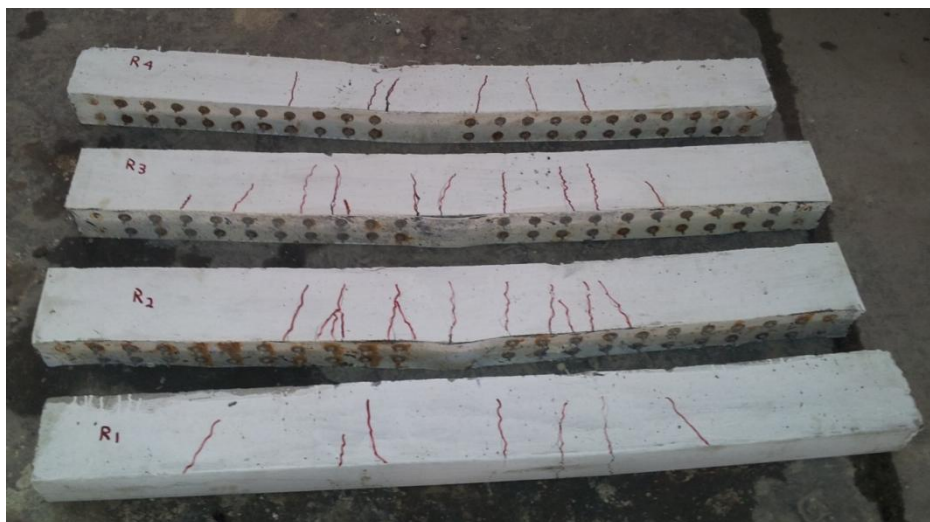
Fig .(7) Failure Mode by Yielding of Steel Plate
