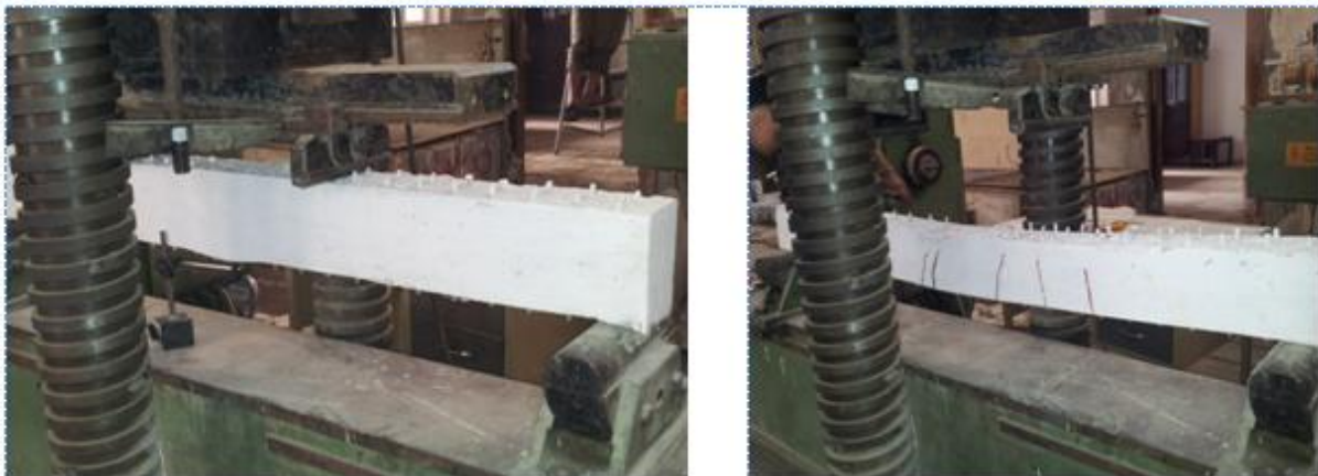
Fig .(8) Beams under Loading Machine
