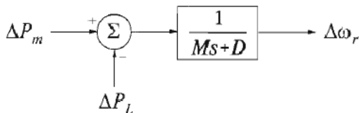
Fig .(4) Transfer function relating speed and power and damping constant [4]
