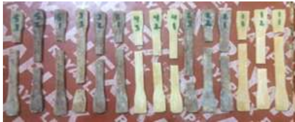
Plate (10) tensile test samples after testing
