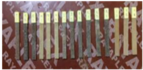
Plate (12) flexural test samples before testing
