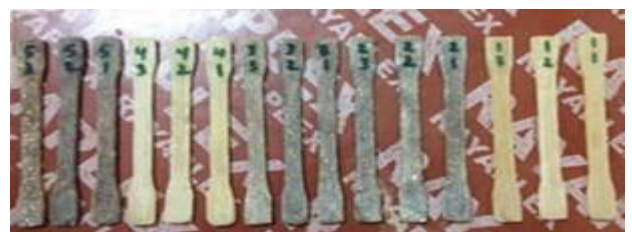
Plate (8) tensile test samples before testing
