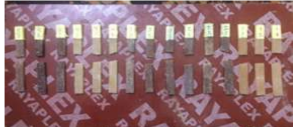
Plate (13) flexural test samples after testing
