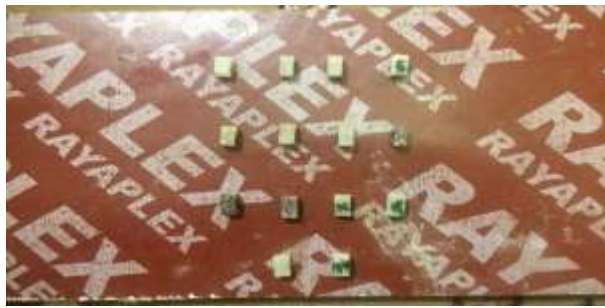
Plate (15) Compression test samples before testing
