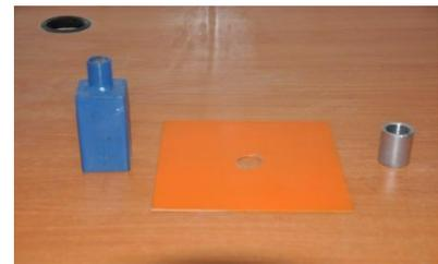
(e) Pile cap for compression test
