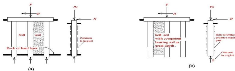
Fig .(1): (a) End-bearing pile. (b) Skin friction-pile
