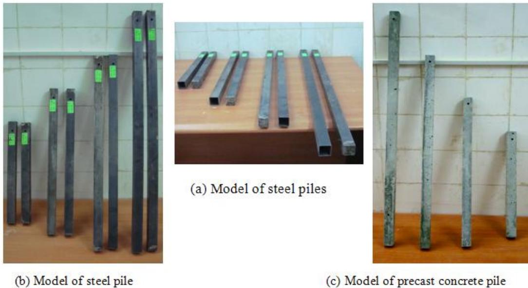
**Fig .(3): model of piles**
