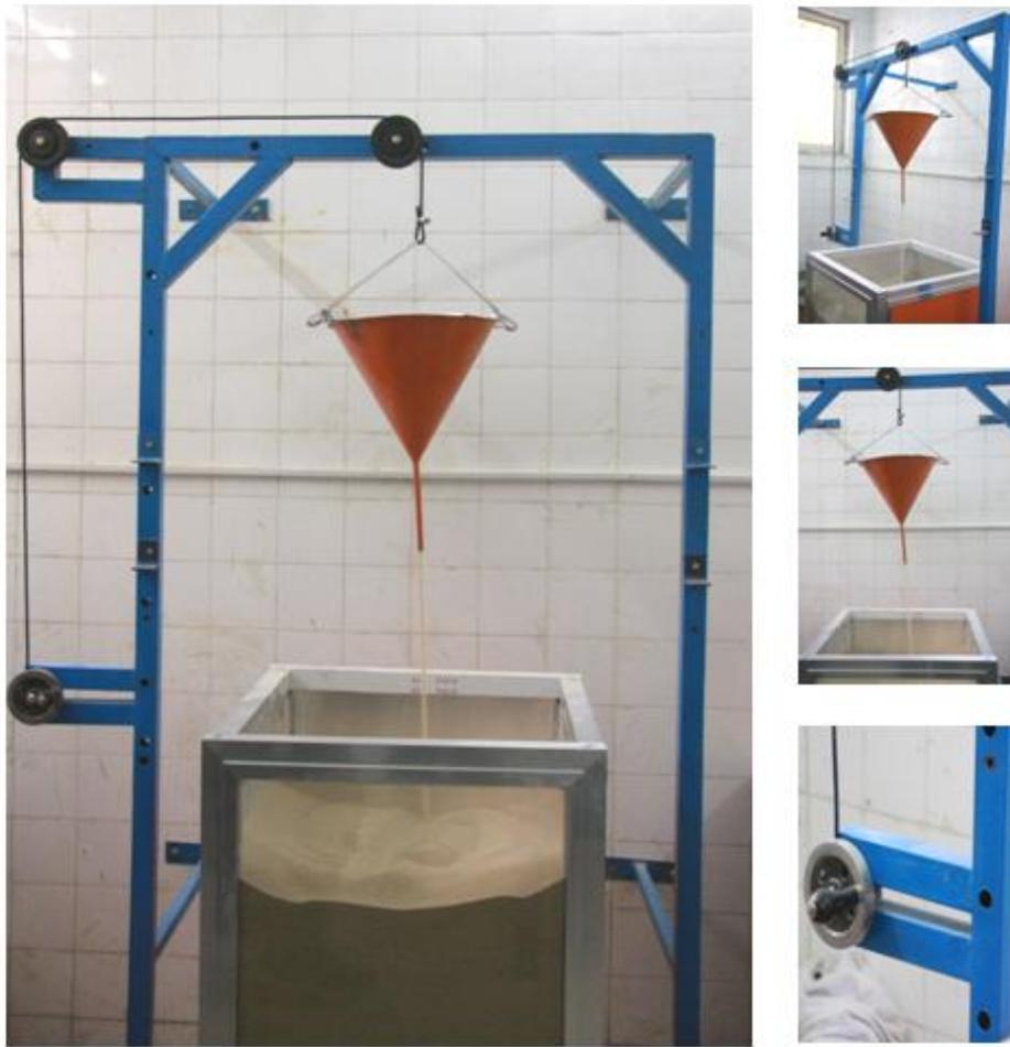
Fig .(6): pouring process of sand
