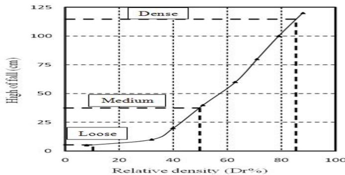
**Fig. (5): Relationship between height of fall and relative density of sand**
