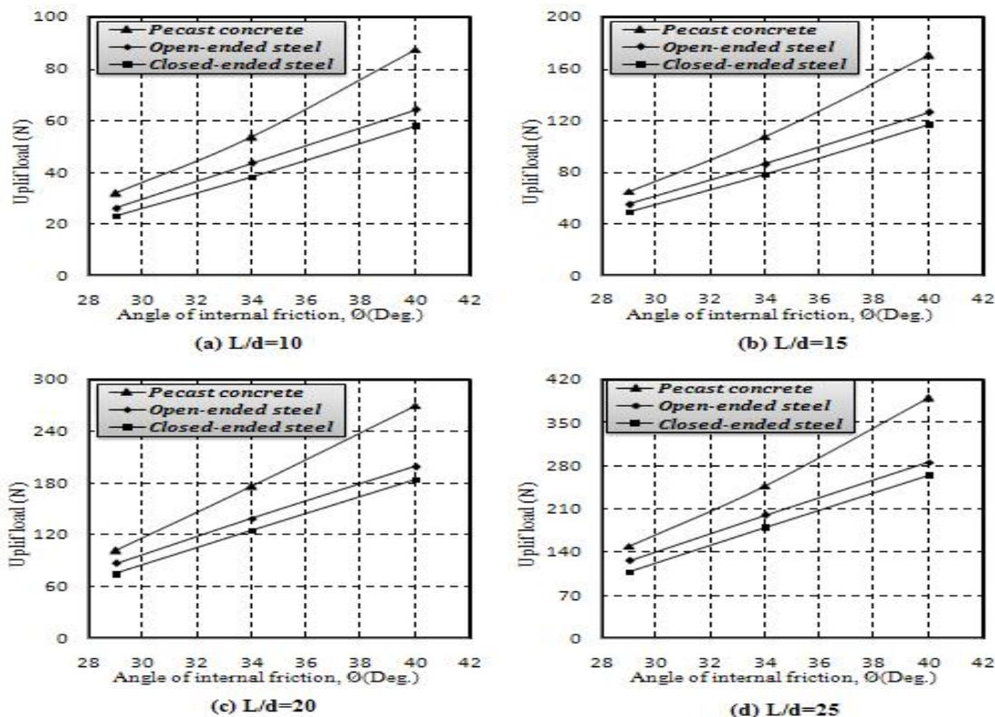
Fig .(11): Relationship between uplift load and angle of internal friction ( $\phi$ ) for three types of piles and different (L/D)
