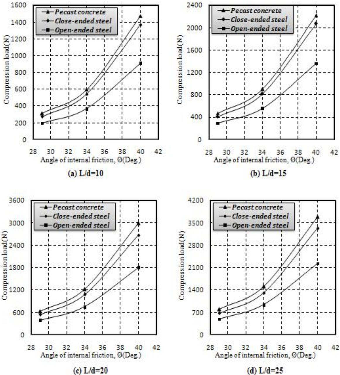
**Fig .(10): Relationship between compression load and angle of internal friction ( $\theta$ ) for three types of model piles and different (L/D) ratio**
