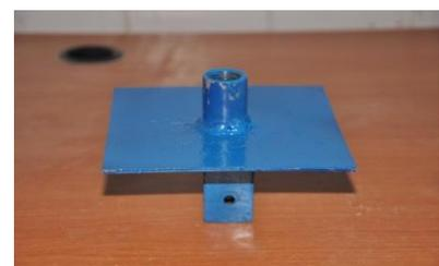
(f) Pile cap for tension test
