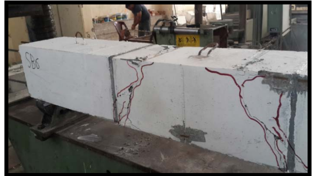
Figure 15. Crack Pattern for specimens SB6
