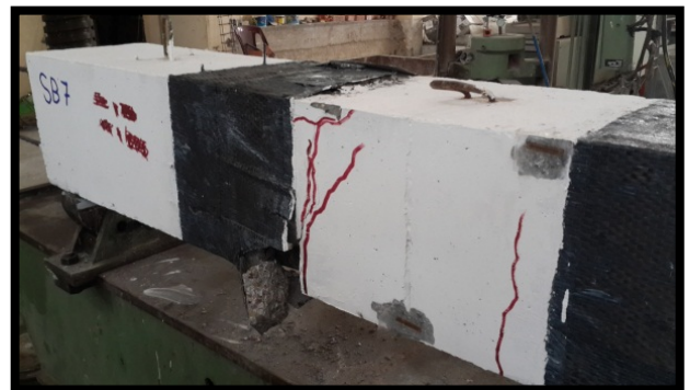
Figure 16. Crack Pattern for specimens SB7
