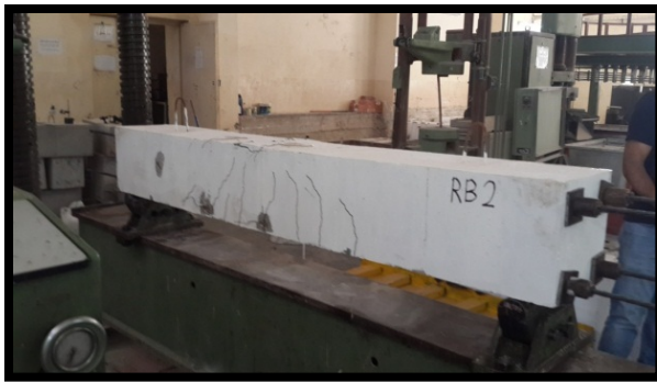
Figure 13. Crack Pattern for specimen RB2
