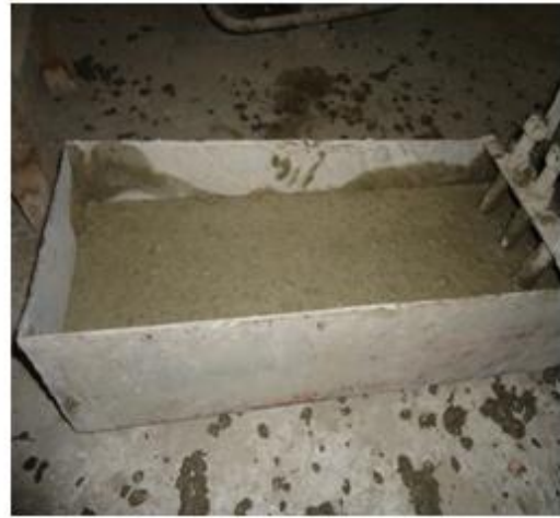
Fig .(3) Flowing of concrete in horizontal section in L-box test of SC
