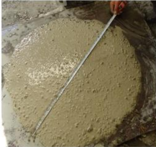
Fig .(2) Spreading concrete in Slump Flow test of SCC
