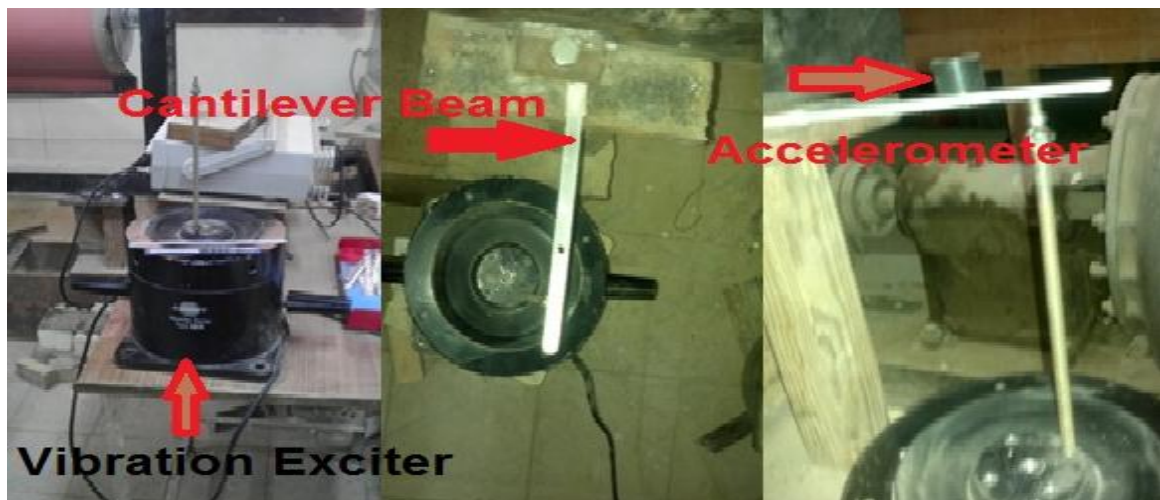
Fig .(3-11) Cantilever beam
