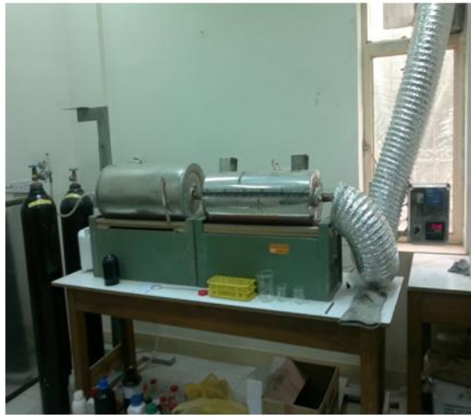
Fig. (3-5) Vacuum Furnace
