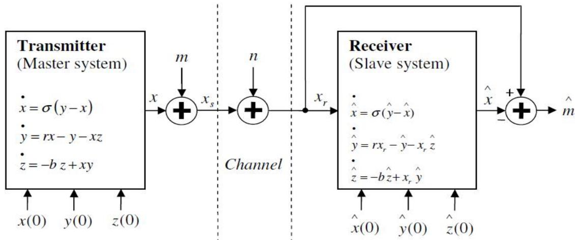
**Fig .(5) The general block diagram of the chaotic communication System based on the chaotic masking concept.**
