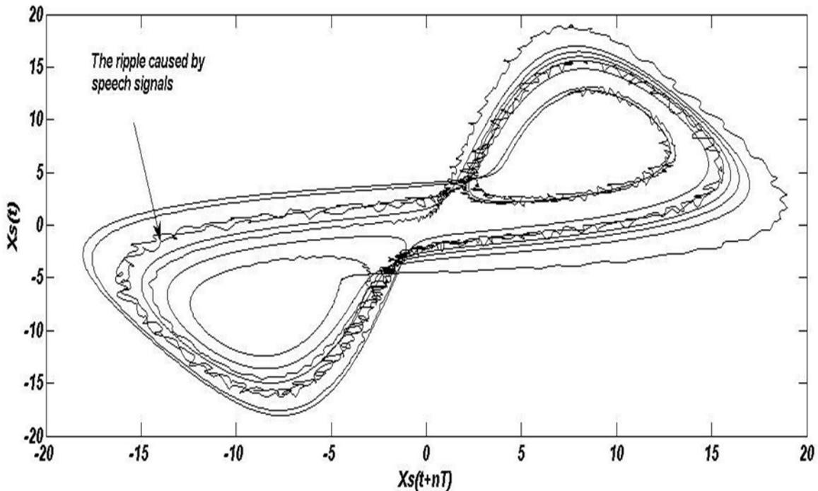
**Fig .(8):**The transmitted signal  $x_s(t)$  plotted in phase space.
