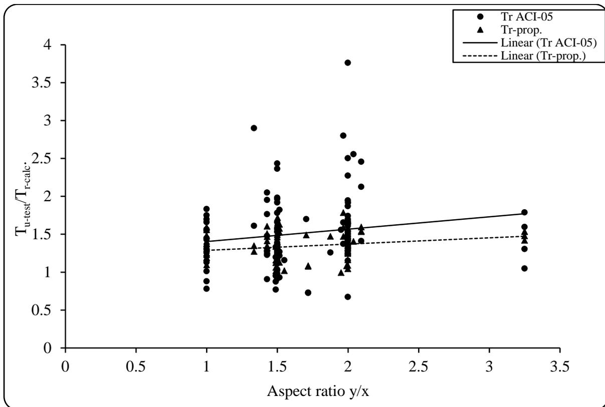
Fig. 2- Influence of aspect ratio  $y/x$  on test results
