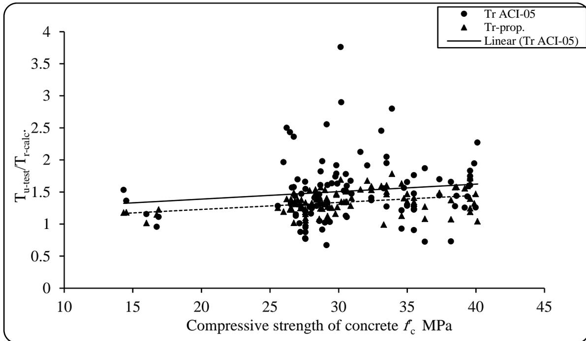
Fig. 1- Influence of compressive strength of concrete  $f_c$  on test results
