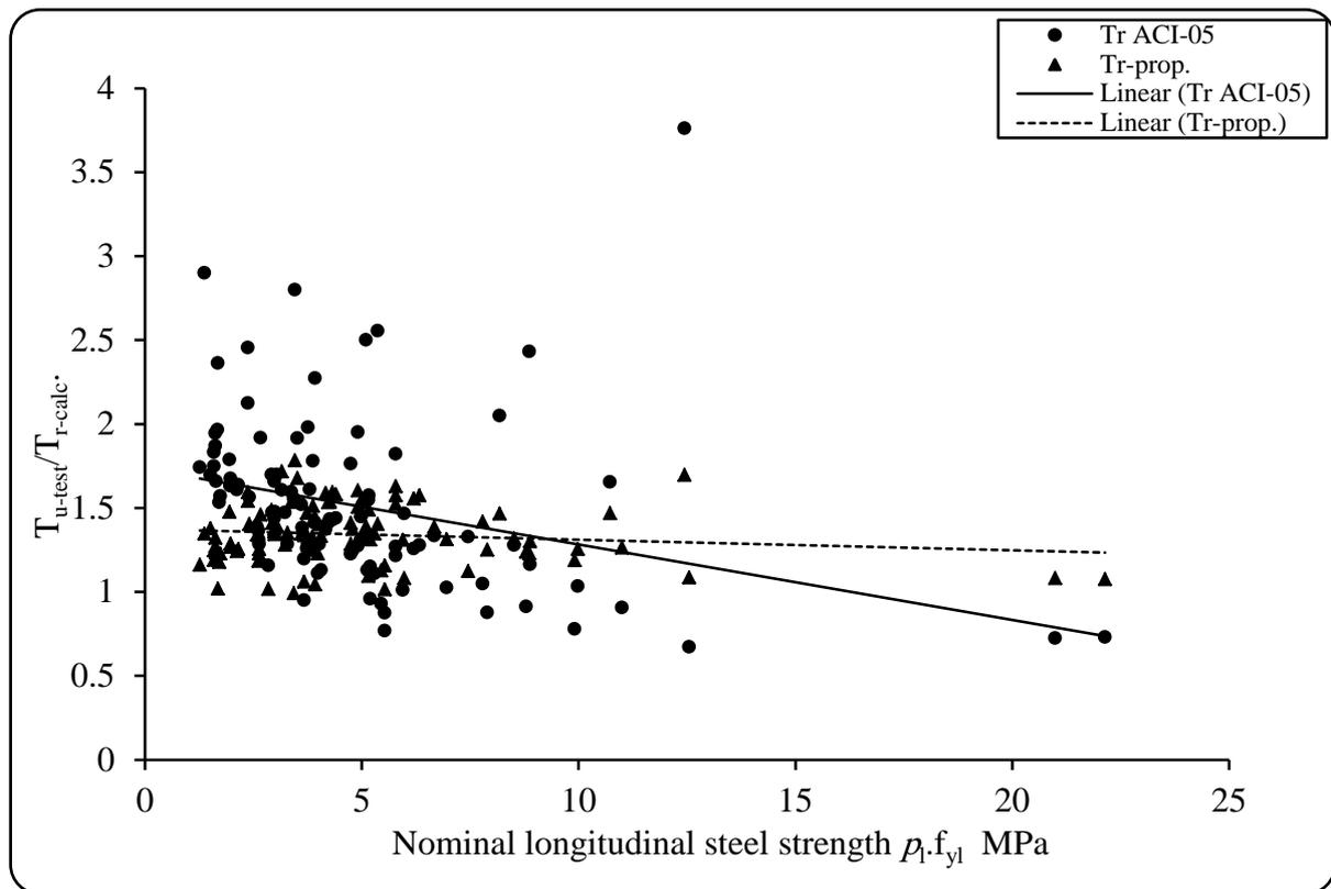
Fig. 5- Influence of nominal longitudinal steel strength  $\rho_l f_{yl}$  on test results
