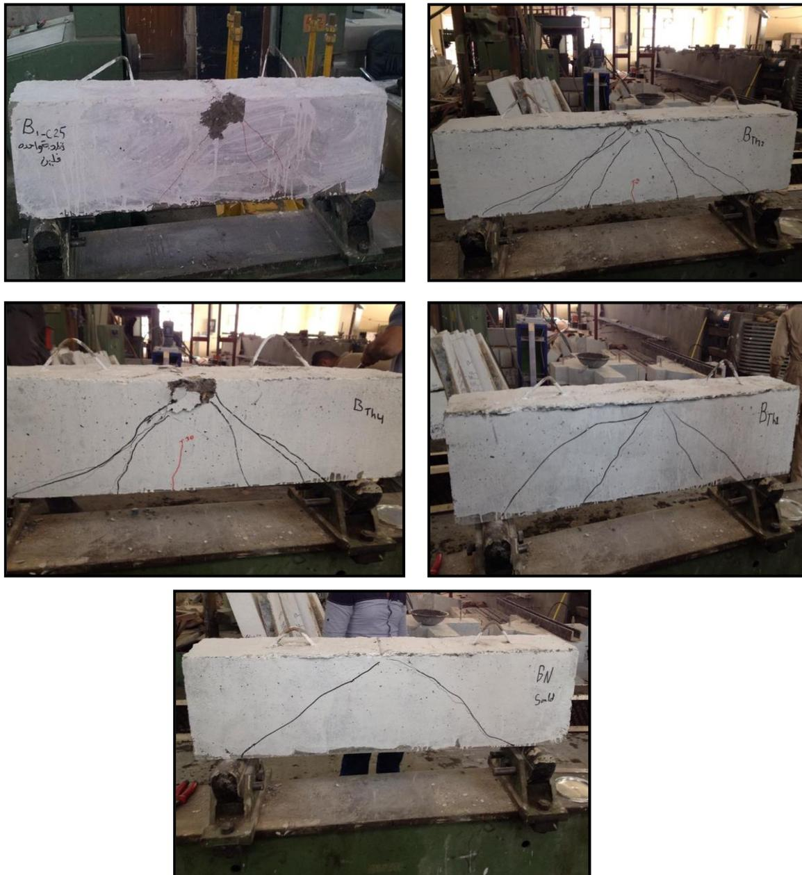
Figure 6. Crack Patterns Tested Beams
