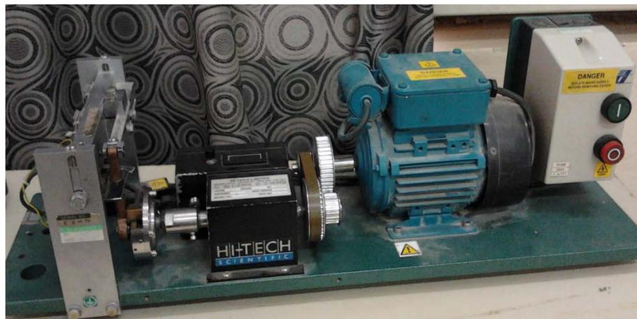
**Fig. 4: Fatigue testing machine.**
