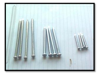
Fig(6): Steel (nail) reinforcement with different lengths related to footing width (Ln/B=11%,14.2%,21.4%) used to stabilize saline soil.
