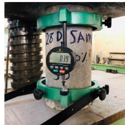
Plate 3. Static modulus of elasticity test
