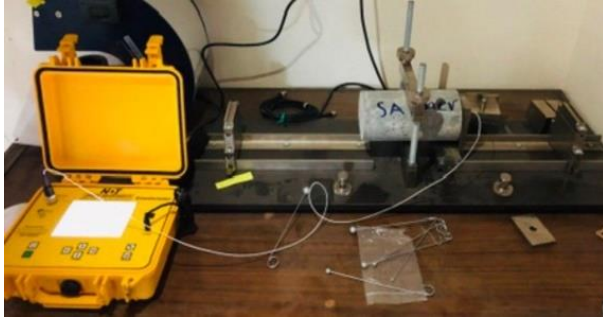
Plate 4. Dynamic modulus of elasticity test
