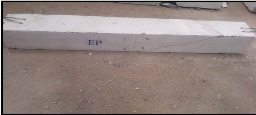
Figure (17), Crack Pattern and Failure Mode of Fibrous ( V_f = 0.8\% ) SCC Beam (Ep)
