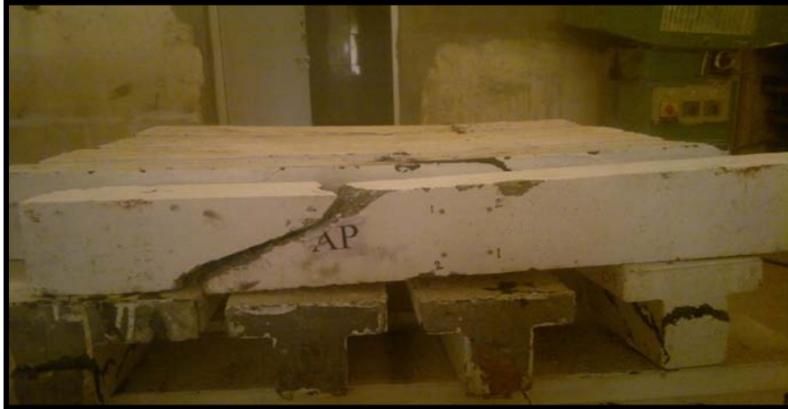
Figure (7), Failure Mode of Normal Strength SCC Beam (Ap)
