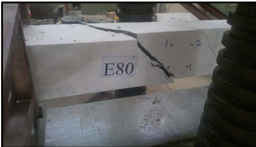
Figure (18), Crack Pattern and Failure Mode of Fibrous ( V_f = 0.8\% ) SCC Beam (E80)
