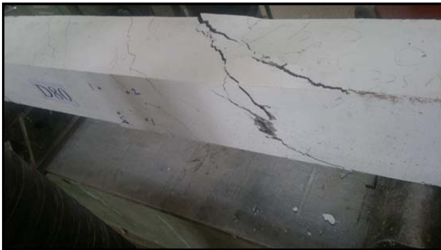
Figure (13), Crack Pattern and Failure Mode of Fibrous ( V_f=0.4\% ) SCC Beam (D80)
