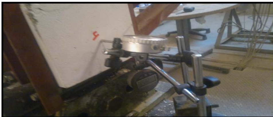
Figure (4), Demec Points and Dial Gauges Arrangement (a) and (b)-demec points arrangement (c) and (d)-dial gages arrangement
