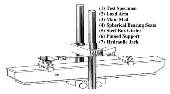
Figure (5): Suggestions of load Arrangement Showing the Test Rig<sup>[5]</sup>.
