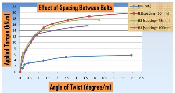
Figure (10): Torque–Twist Behavior of Composite Concrete-Steel Beams
