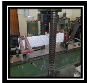
Figure (12): Failure of Reference (BN) Mode of Specimen
