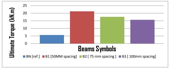
Figure (9): Load carrying capacity of the tested beams
