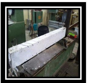
**Finger (13): Crack Pattern and Failure**
