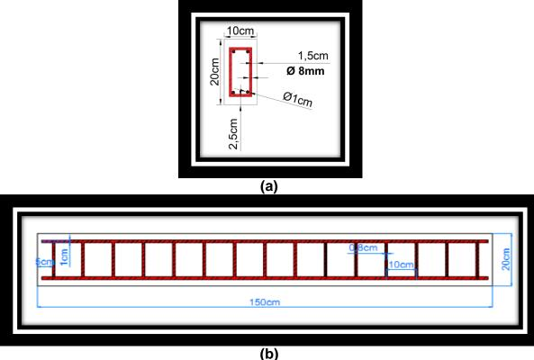
(D) Figure (3): Defiles of Beams Reinforcement (a) Cros Section of Steel Reinforcement. (b) Reinforcement Profile along the Beam.
