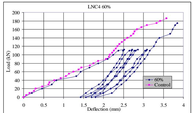
Figure 9 Load- deflection response for corbel LNC4 (60% loading level).
