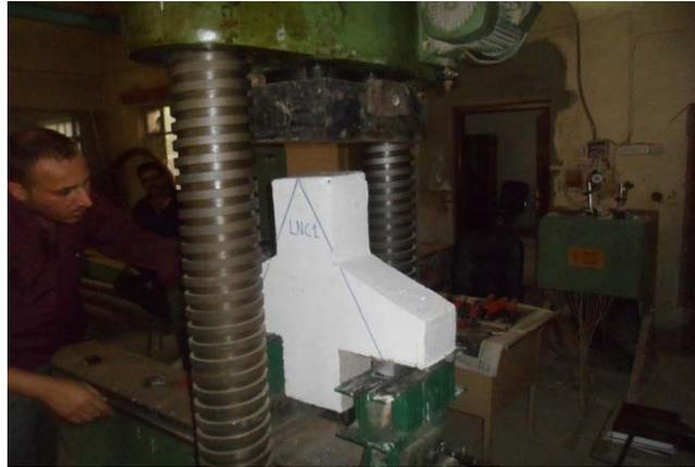
**Plate 1 Corbel specimen Setup**
