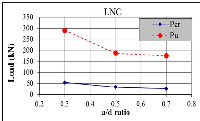
**Figure 2 Effect of  $a/d$  ratio on cracking and ultimate loads for LNC corbels**
