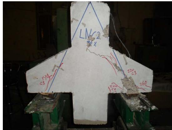
**Plate 3 Crack pattern for corbel LNC2 (repeated load 90%) after testing**
