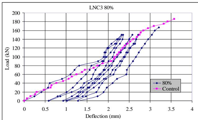
Figure 8 Load- deflection response for corbel LNC3 (80% loading level).
