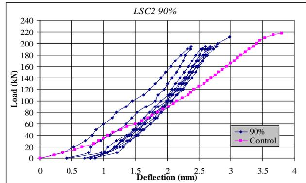
Figure 11 Load- deflection response for corbel LSCC2 (90% loading level).
