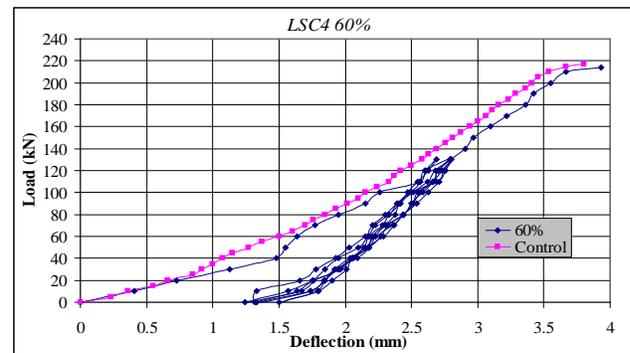
Figure 13 Load- deflection response for corbel LSCC4 (60% loading level).
