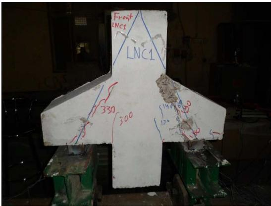
**Plate 2 Crack pattern for corbel LNC1 (monotonic load) after testing**
