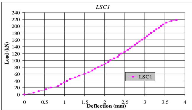
Figure 10 Load- deflection response for corbel LSCC1 (monotonic loading).
