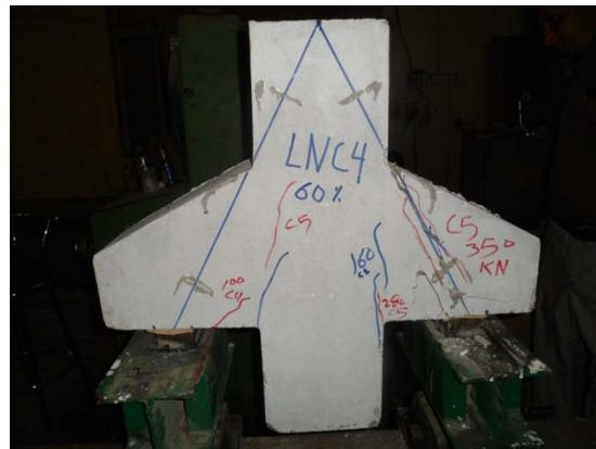
**Plate (5) Crack pattern for corbel LNC4 (repeated load 60%) after testing**
