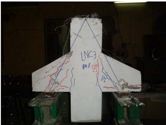
**Plate 4 Crack pattern for corbel LNC3 (repeated load 80%) after testing**
