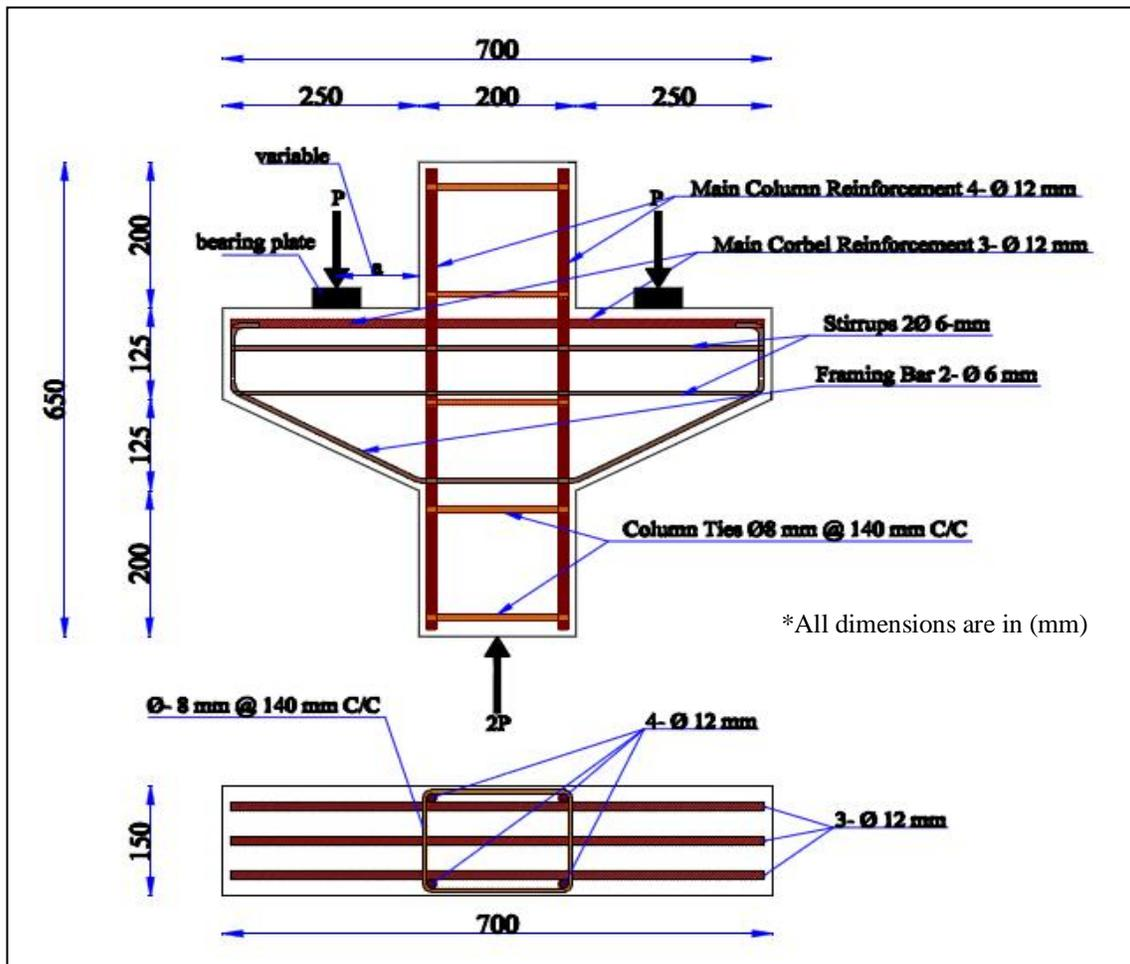
Figure 1 Details of tested corbel.
