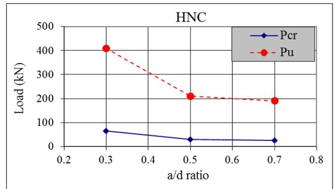
**Figure 3 Effect of  $a/d$  ratio on cracking and ultimate load of HNC corbels**
