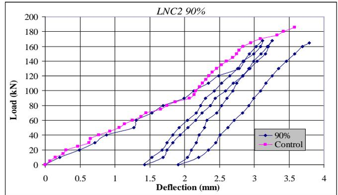
Figure 7 Load- deflection response for corbel LNC2 (90% loading level).
