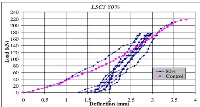
Figure 12 Load- deflection response for corbel LSCC3 (80% loading level).
