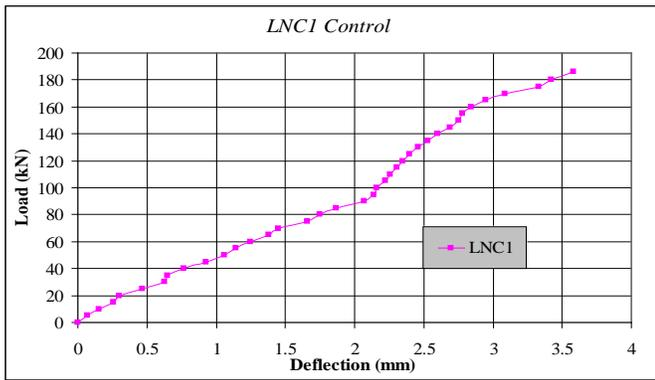
Figure 6 Load- deflection response for control corbel LNC1 (monotonic loading).
