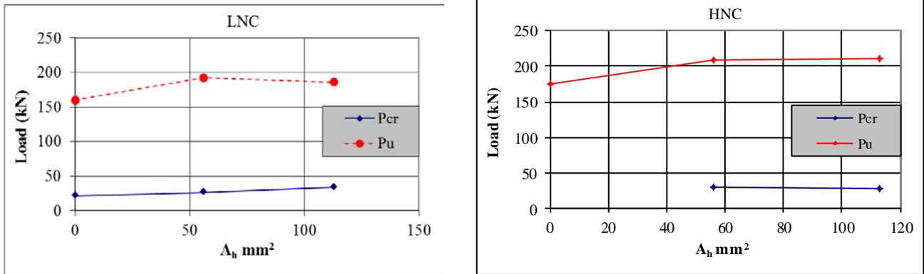
Figure 4 Effect of horizontal stirrups on the ultimate load of corbels with (a/d =0.5)
