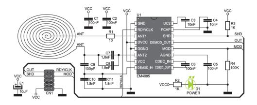
Figure (3) schematic circuit of RFID
