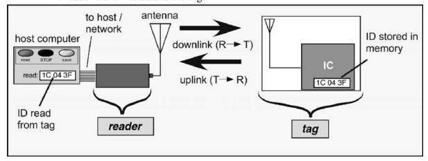
Figure (1) Basic Operations of RFID [3]
