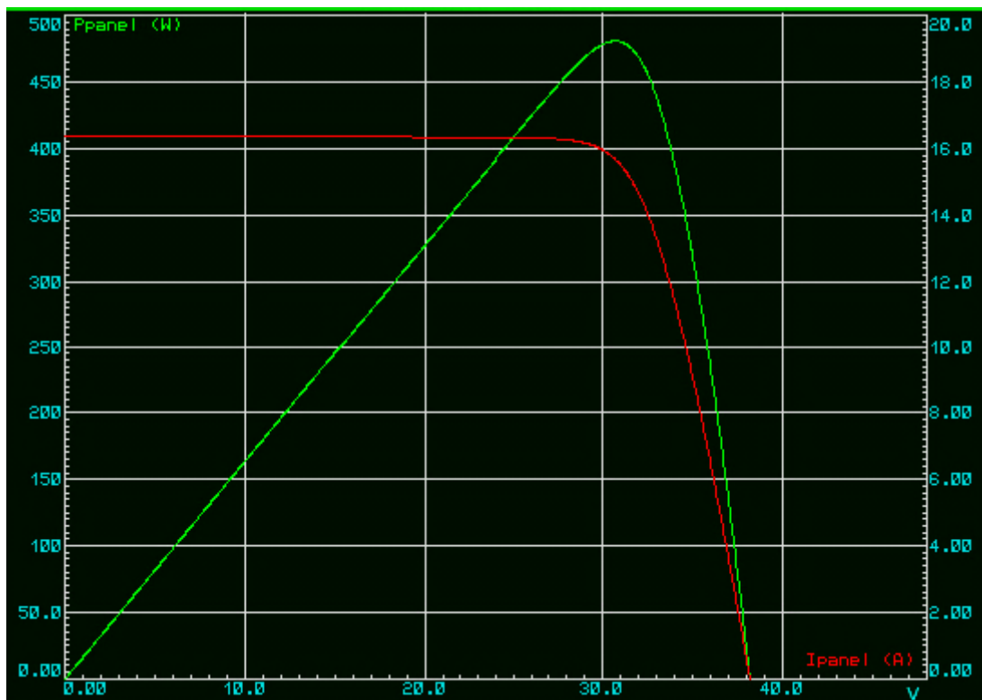
Figure 9. PV output current, power versus the output voltage to a variable load
