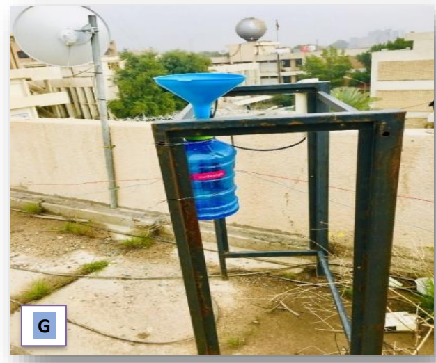
Figure 1. (A) Gutters. (B) Downspouts.(C) Storage tanks (D) Pipe mesh. (E) Downspouts and gutter. (F) First flush. (G) Rain gauge.
