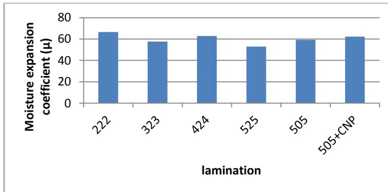
Fig. (5) Moisture Expansion Coefficient ( $\beta$ ) for each lamination
