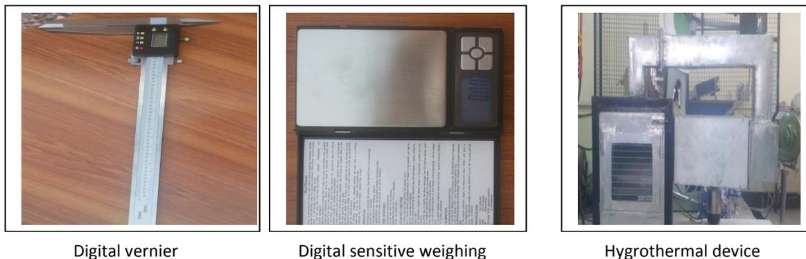
Fig. (2) The equipment used in moisture absorption test
