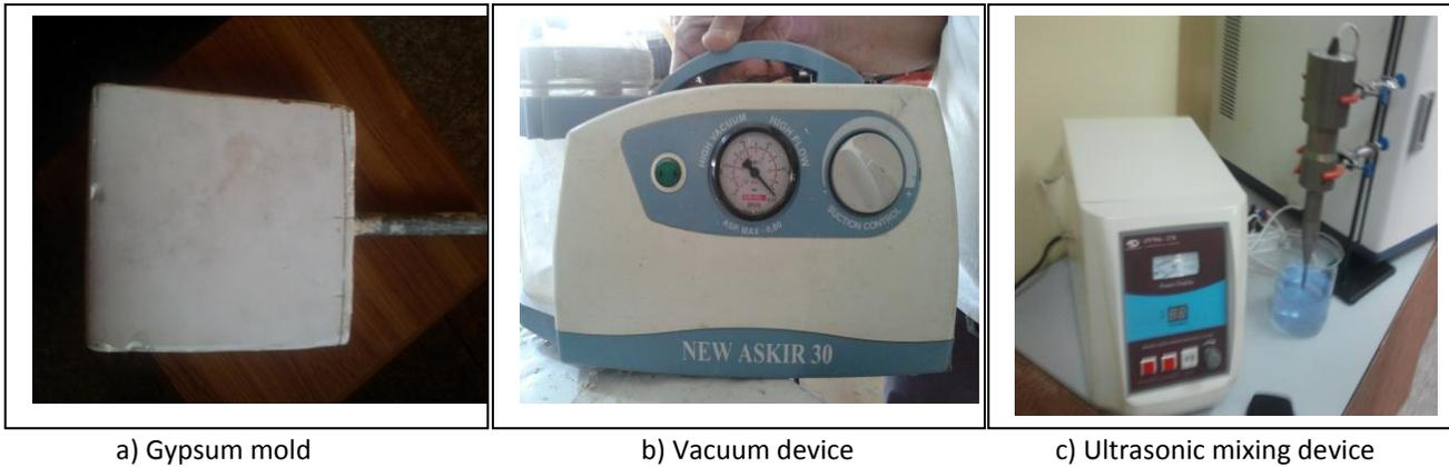
Fig. (1) Equipment and tools used in manufacturing A-K socket lamination
