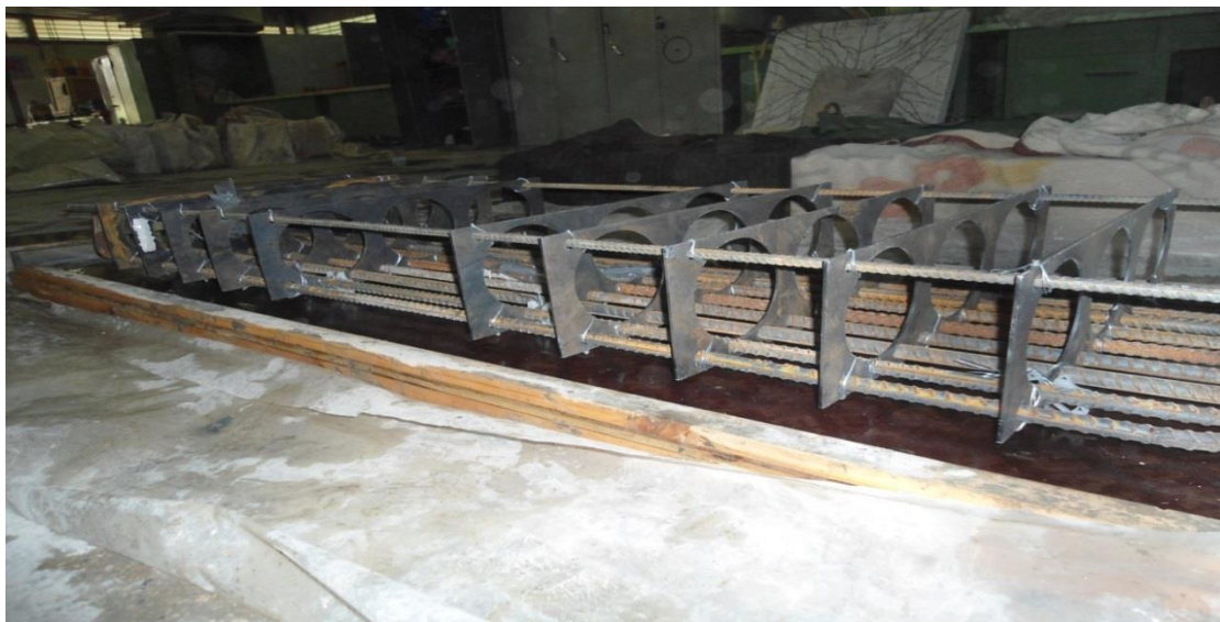
Fig. 4 Preparation the mold specimen and placing the reinforcement
