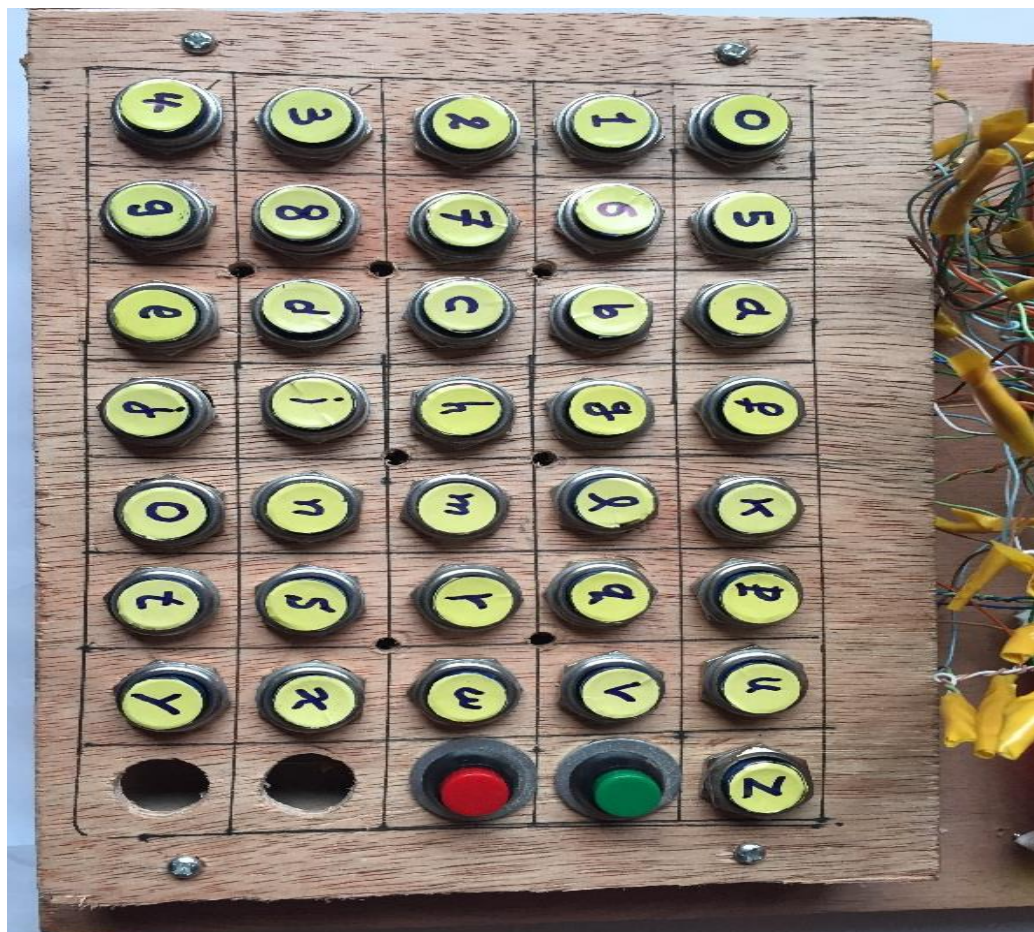
Figure 2. keypad designed for the proposed system.
