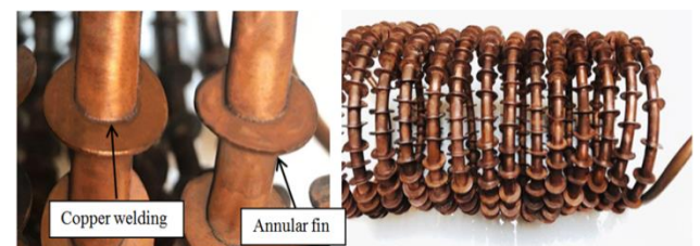
Figure 8. Annular Fins in the Helical Coil
