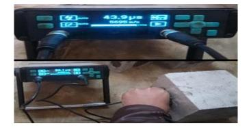
Figure 5. Ultrasonic test
