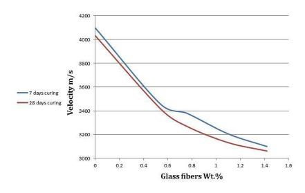
Figure 9. Effect of random glass fibers addition to mortar on velocity
