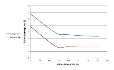
Figure 6. Effect of random glass fibers addition on the water absorption of mortar
