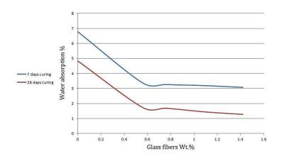
Figure 7. Effect of glass fiber layers addition on the water absorption of mortar
