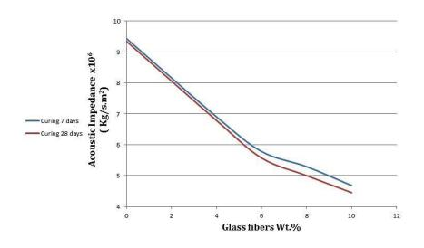
Figure 13. Effect of glass fibers layers addition on acoustic impedance
