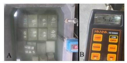
Figure 4. Curing at (a) controlled temperature and (b) controlled humidity
