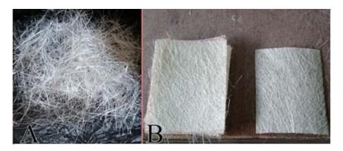
Figure 2. A: Random glass fibers, B: Glass fibers layers.
