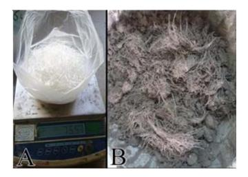
Figure 3. (a) Glass fibers weighing, (b) preparation of glass fibers mortar.
