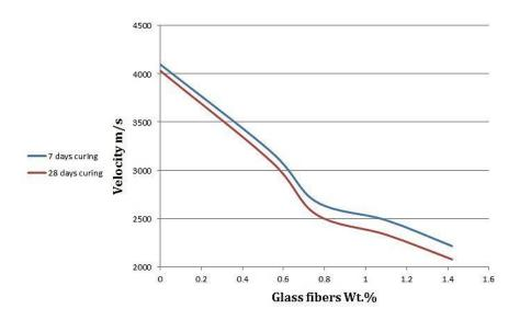
Figure 10. Effect of glass fibers layers addition to mortar on velocity
