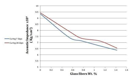
Figure 12. Effect of random glass fibers addition on acoustic impedance
