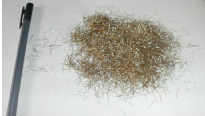
Fig .(1) Sample of micro steel fibers used in present investigation
