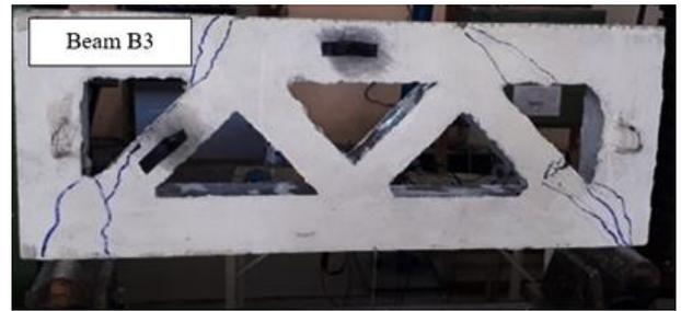
**Figure 8.** Mode Failure of Specimen B3
