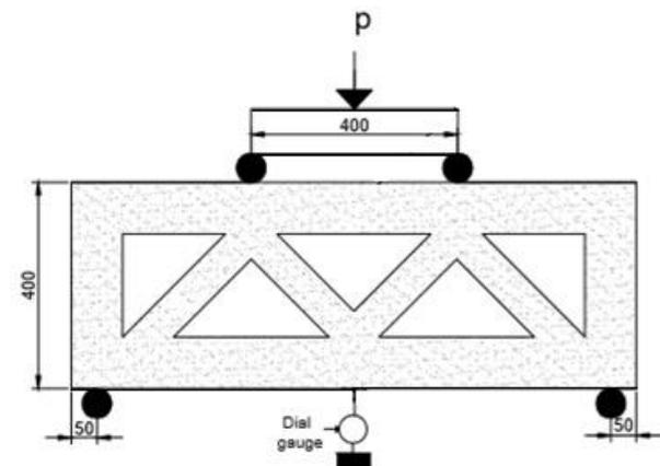
**Figure 4.** Testing Set-up of Coupled Beam Specimens
