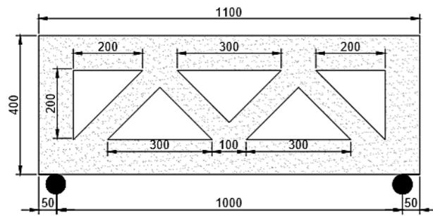
**Figure 1.** Details of Coupled Beams
