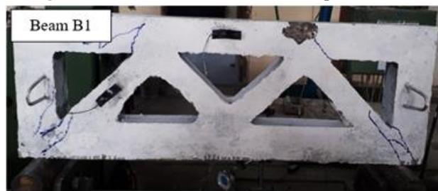
**Figure 6.** Mode Failure of Specimen B1
