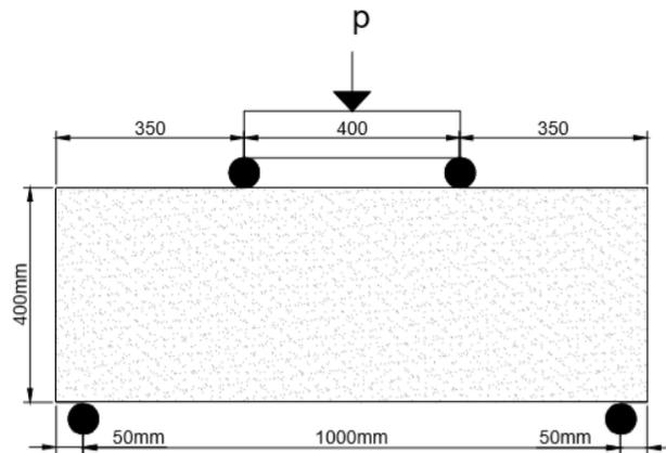
**Figure 3.** Testing Set-up of Reference Specimen RN
