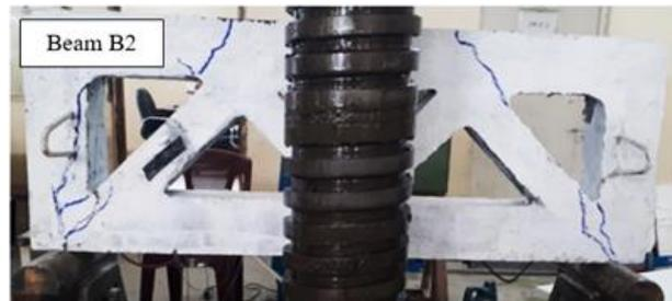
**Figure 7.** Mode Failure of Specimen B2
