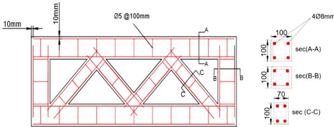
**Figure 2.** Reinforcement Details of Coupled Beams
