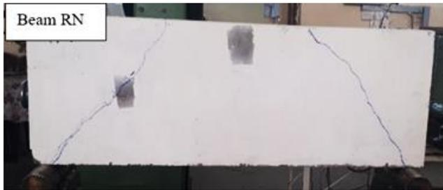
**Figure 5.** Mode Failure of Reference Specimen RN
