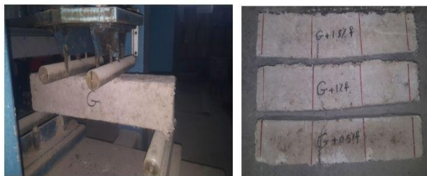
Figure 6. Beams before and after Failure
