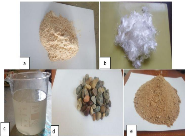
Figure 1. Materials used for research (a) Metakaolin (b) Polypropylene fiber (c) Alkaline Liquid (d) coarse aggregate (e) fine aggregate.
