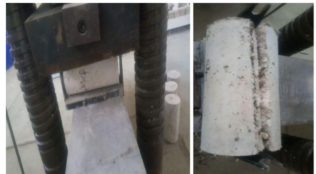
Figure 4. GPC Cylinder before and after testing
