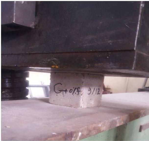
Figure 2. GPC Cube at Test Machine
