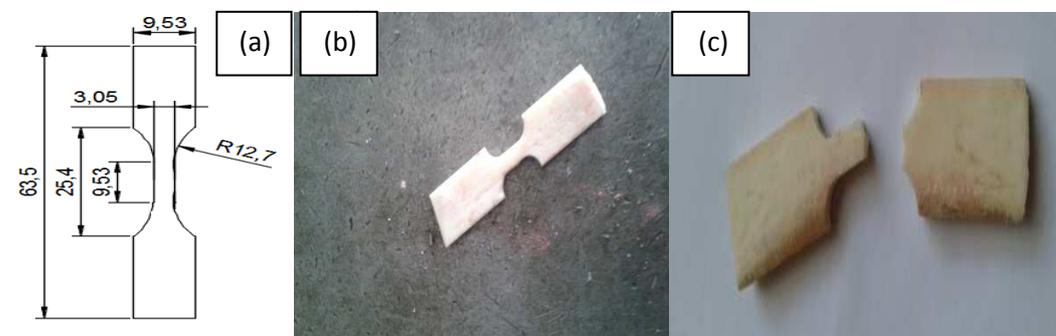
Figure 2. (a) The dimension of the specimen of tensile test for the bone according ASTM D638 [7]. Type V, all dimensions in mm, (b) and (c) The tensile test specimen of the human bone before and after the failure respectively.
