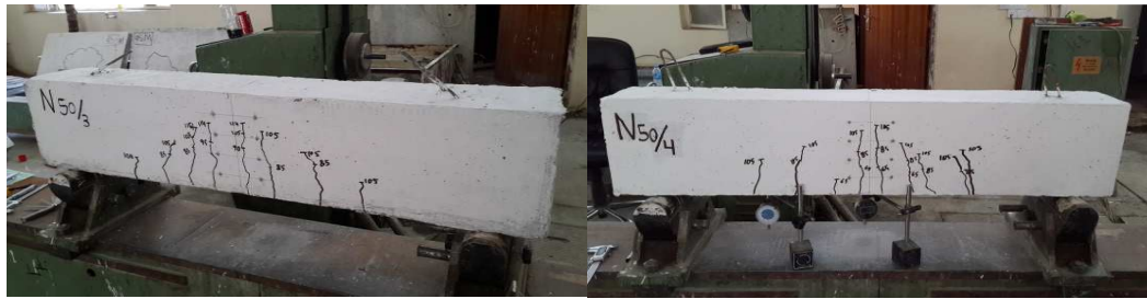
(c) Recycled aggregate with steel fiber (d) Recycled aggregate without steel fiber
