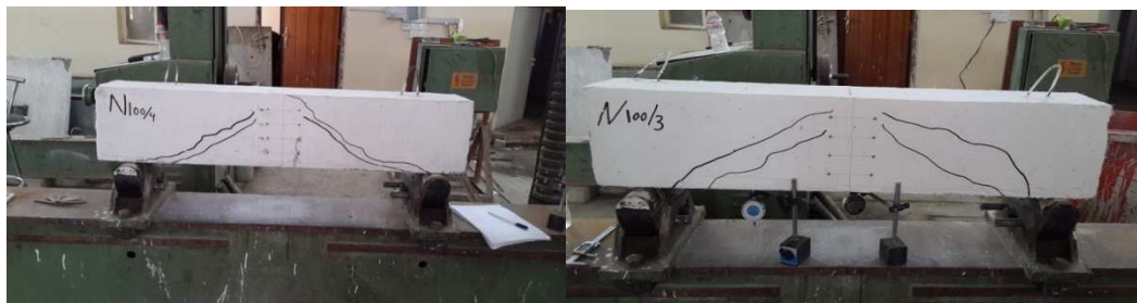
(g) Recycled aggregate with steel fiber (h) Recycled aggregate without steel fiber
