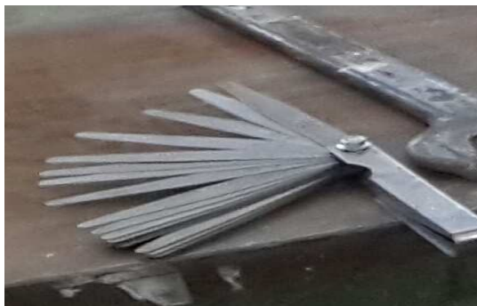
Figure 9: Crack width measurement
