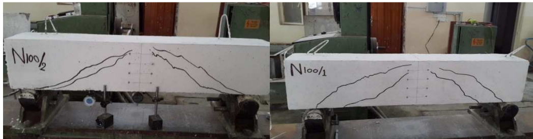
(e) Natural aggregate with steel fiber (f) Natural aggregate without steel fiber
