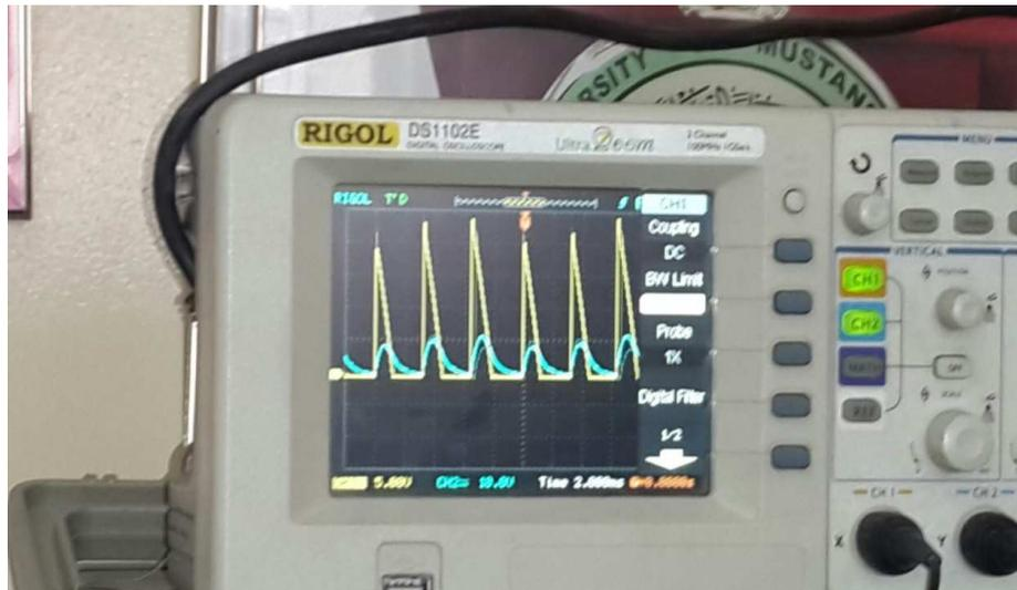
Fig. (10) The voltage and current waveforms for ( $\alpha \approx 95^\circ$ ) Time scale= 2ms, Voltage scale, ch1=5V, ch2=10V
