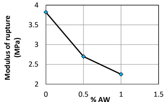
**Figure 6.** Effect of Aluminum waste on modulus of rupture
