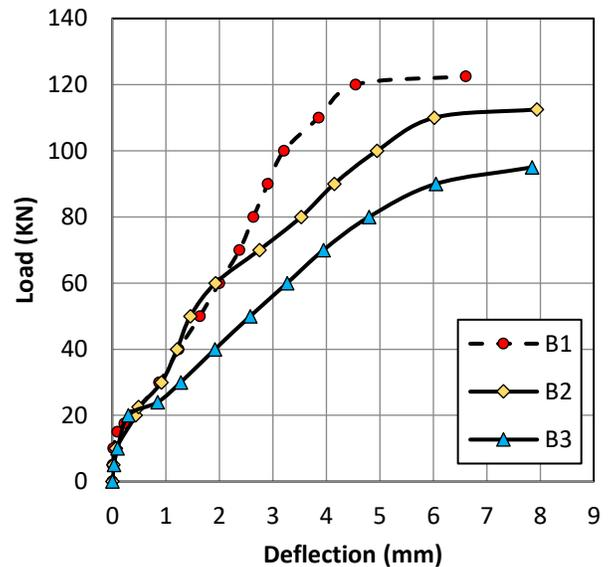
**Figure 11.** Load-mid span deflection of tested beams
