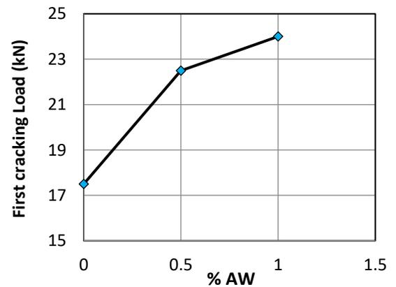
**Figure 8.** Aluminum waste fraction versus first cracking load
