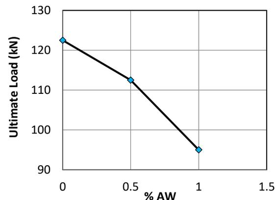
**Figure 9.** Aluminum waste fraction versus ultimate load
