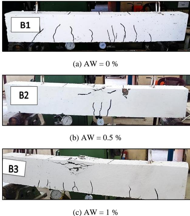
Figure 12. Crack patterns of tested beams
