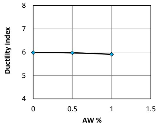
Figure 13. Effect of aluminum waste on ductility index
