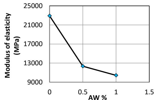
**Figure 7.** Effect of Aluminum waste on the modulus of elasticity
