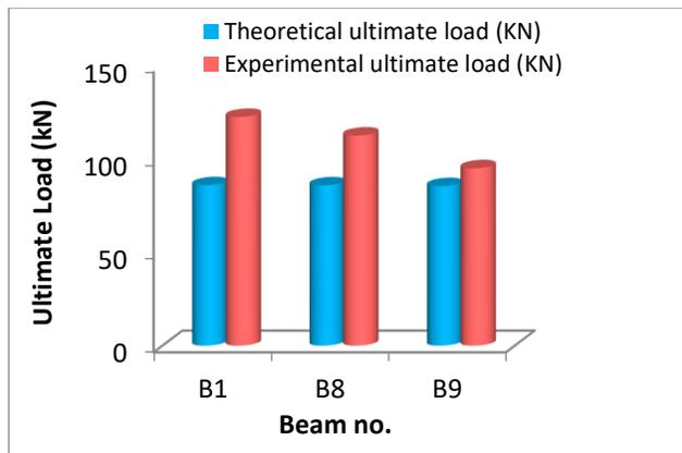
**Figure 10.** Percent of increasing in experimental ultimate load compared to the theoretical value of tested beams
