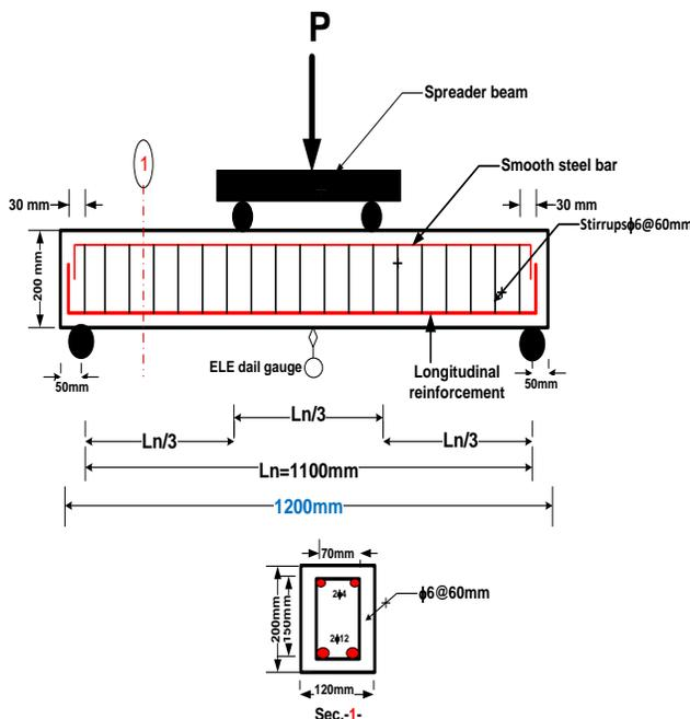
Figure. 3 Details and test setup of reinforced beams
