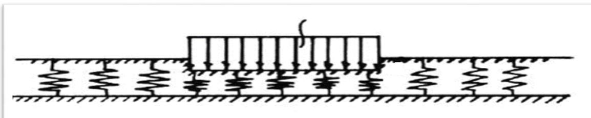
Figure -1 Surface displacement of Winkler model to uniform.<sup>[7]</sup>
