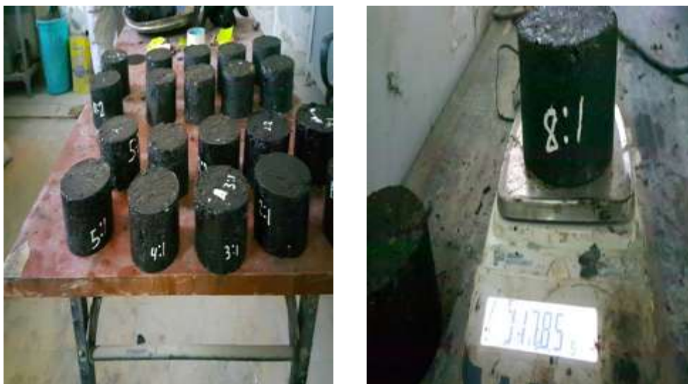
Plate (5) Marshal Test Specimen
