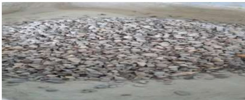
Plate(4) Recycled coarse aggregate of 10 mm maximum size
